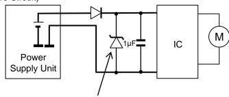
Add the zener diode in parallel with bypass capacitance
