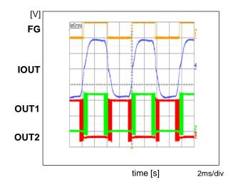
Condition:  $V_{CC} = 12 \; V, \; PWMI = 100\% \; duty \; , \; Cvcc = 1 \; \mu F$
