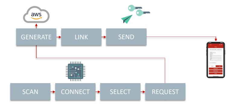
Then the App will transfer the provisioning Keys over BLE to the Device
