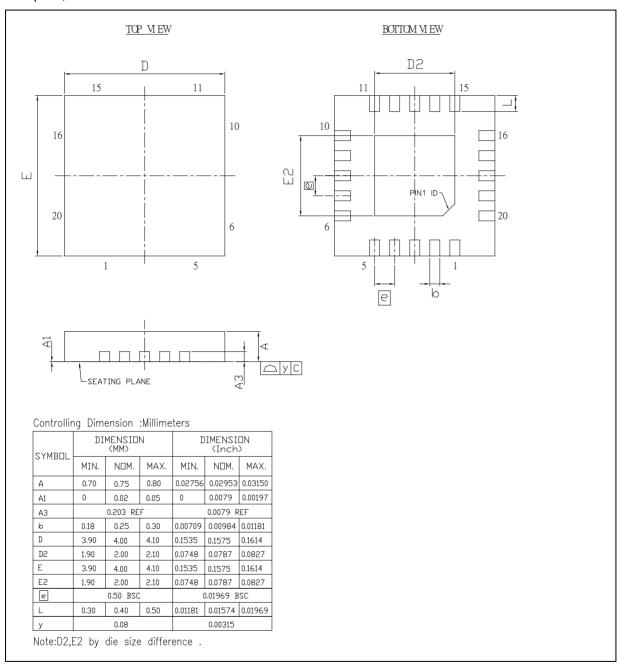
NAU8318 20 pin QFN Package Specification
