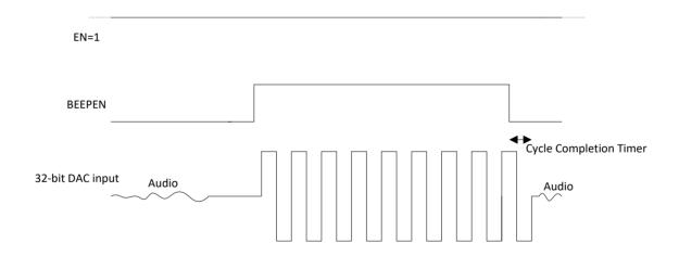
Figure 8 BEEP Timing during operation
