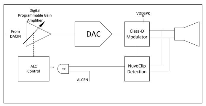
Figure 12 ALC Control Loop Block Diagram
