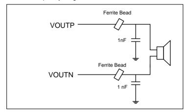
Figure 14 NAU8318 Speaker Connections with Ferrite Bead Filters
