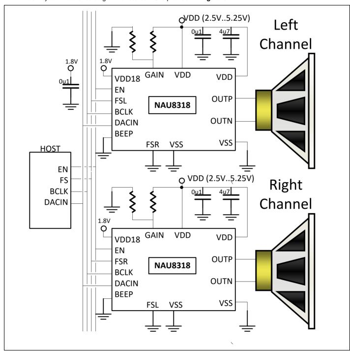
Figure 3 NAU8318 Simplified System Diagram
