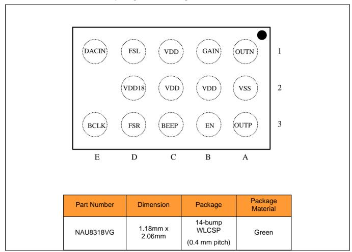
Figure 1 Pin Configuration of WLCSP14 NAU8318 (TOP VIEW)
