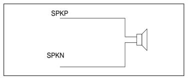
Figure 13 NAU8318 Speaker Connections without Filter
