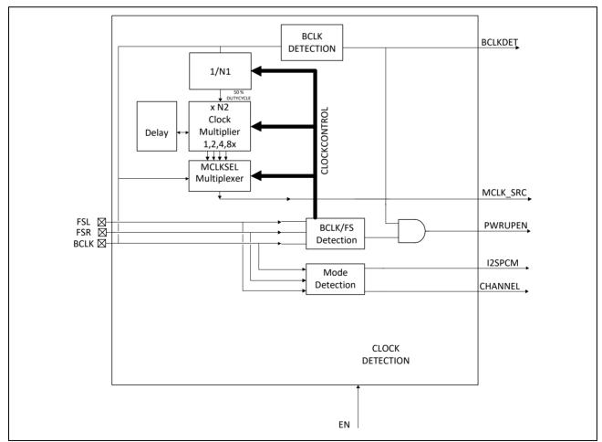
Figure 10 NAU8318 Clock Detection Circuit
