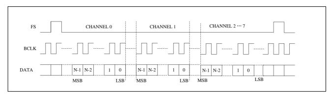
Figure 18 PCM Time Slot Audio Data
