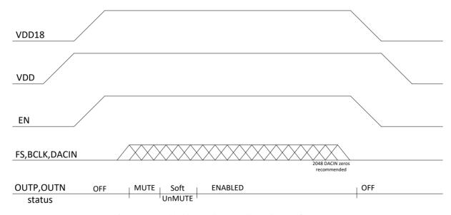
Figure 9 NAU8318 Power Up & Down Sequence
