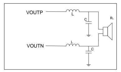
Figure 15 NAU8318 Speaker Connections with LC Filters
