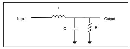
Figure 16 NAU8318 Speaker Connections with Low-Pass Filters
