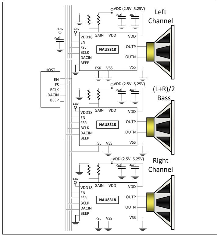
Figure 4 NAU8318 System Diagram for 2.1 sound
