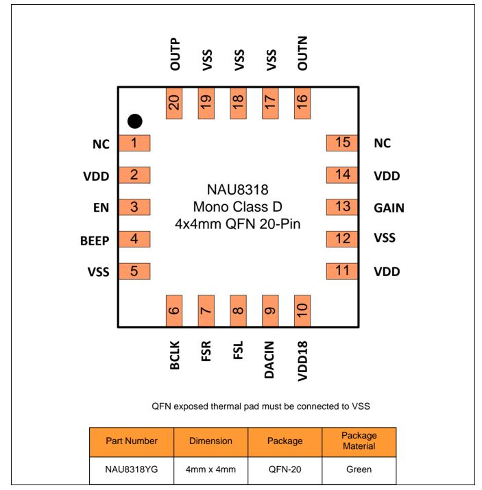
Figure 2 Pin Configuration of QFN20 NAU8318
