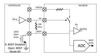
Figure 6 BEEP Pin Configurations & Settings
