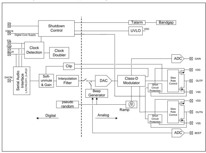
Figure 5 NAU8318 Block Diagram
