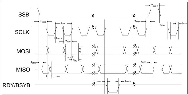
Figure 11-2 SPI Timing
