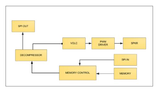
Figure 9-1 ISD2100 Signal Path
