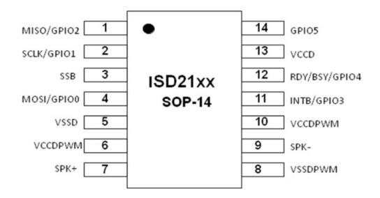
Figure 4-2 ISD2100 SOP14 Pin Configuration
