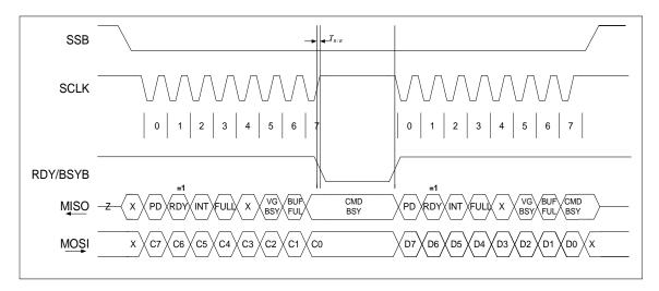
Figure 8-2 RDY/BSYB Timing for SPI Writing Transactions.
