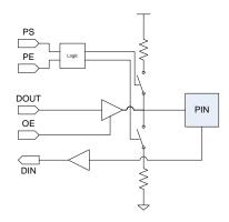
Figure 6-1 GPIO Structure
