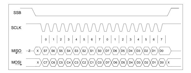
Figure 8-1 SPI Data Transaction.
