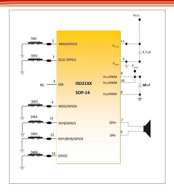
Figure 12-2 ISD2100 Application Diagram Stand-Alone Mode
