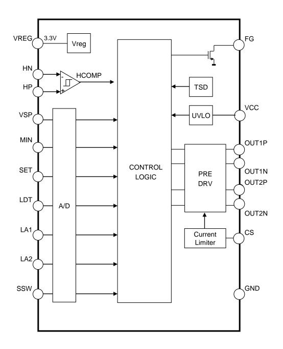
Notes: This block diagram is for explaining functions. Part of the block diagram may be omitted, or it may be simplified.
