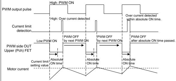
Normal mode(Motor speed > FG frequency 6.67Hz) :Current limit setting voltage = 150mV (Vcs1) Start up mode(Motor speed < FG frequency 6.67Hz) :Current limit setting voltage = 90mV (Vcs2)
