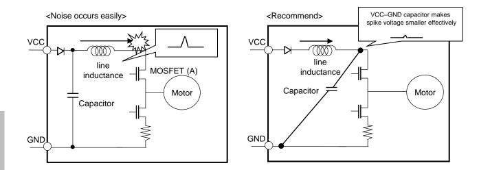
At motor driving, Vcc current flows to MOSFET.
