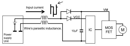
The current peak is reduced according to adding in series with bypass capacitance.
