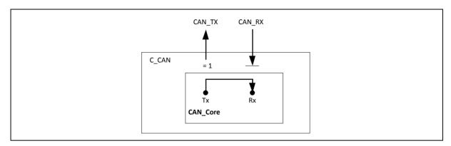
Figure 6.23-4 CAN Core in Loop Back Mode Combined with Silent Mode
