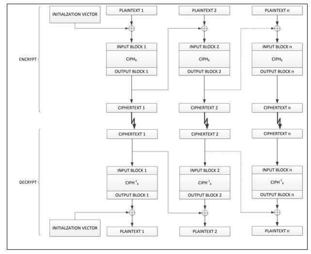
Figure 6.26-4 Cipher Block Chaining Mode
