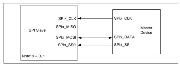
Figure 6.17-11 SPI Half-Duplex Slave Mode Application Block Diagram
