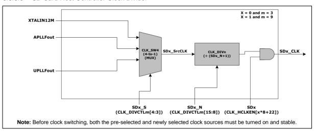
Figure 6.3-3 SD Card Host Controller Clock Divider Block Diagram
