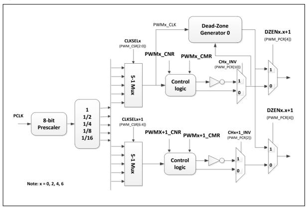
Figure 6.10-1 Two Channels of PWM in One Pair
