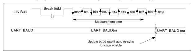
Figure 6.14-22 LIN Sync Field Measurement
