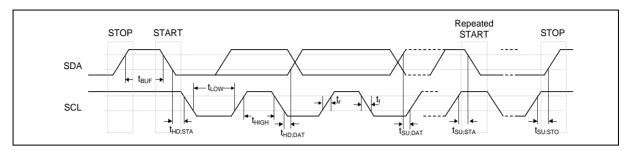
Figure 6.16-2 I<sup>2</sup>C Bus Timing
