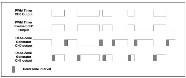
Figure 6.10-5 Paired PWM Output with Dead-Zone Generation Operation
