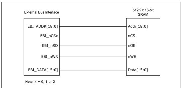
Figure 6.6-2 Connection of 16-bit EBI Data Width with 16-bit Device in Separate mode
