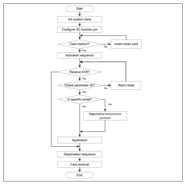
Figure 6.15-7 Basic Operation Flow
