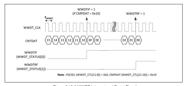
Figure 6.12-6 WWDT Interrupt and Reset Signals
