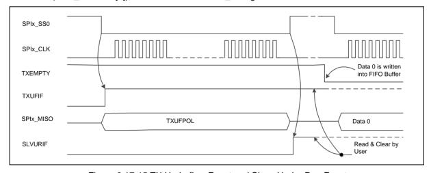
Figure 6.17-15 TX Underflow Event and Slave Under Run Event
