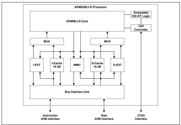
Figure 6.1-1 ARM926EJ-S™ Block Diagram
