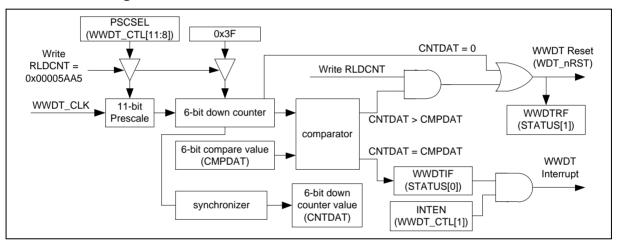
Figure 6.12-1 WWDT Block Diagram
