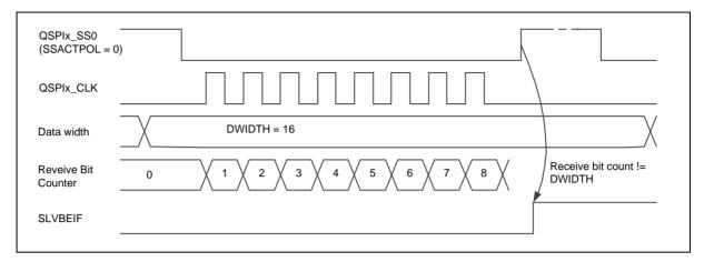
Figure 6.18-24 Slave Mode Bit Count Error
