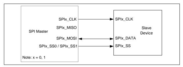
Figure 6.17-10 SPI Half-Duplex Master Mode Application Block Diagram
