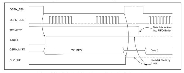
Figure 6.18-21 TX Underflow Event and Slave Under Run Event
