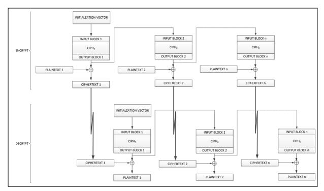
Figure 6.26-6 Output Feedback Mode
