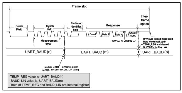
Figure 6.14-23 UART BAUD Update Sequence in AR mode if SLVDUEN is 1
