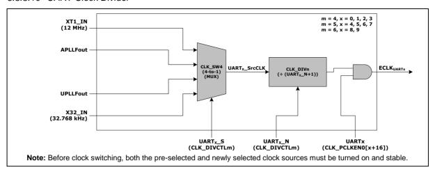
Figure 6.3-10 UART Clock Divider Block Diagram
