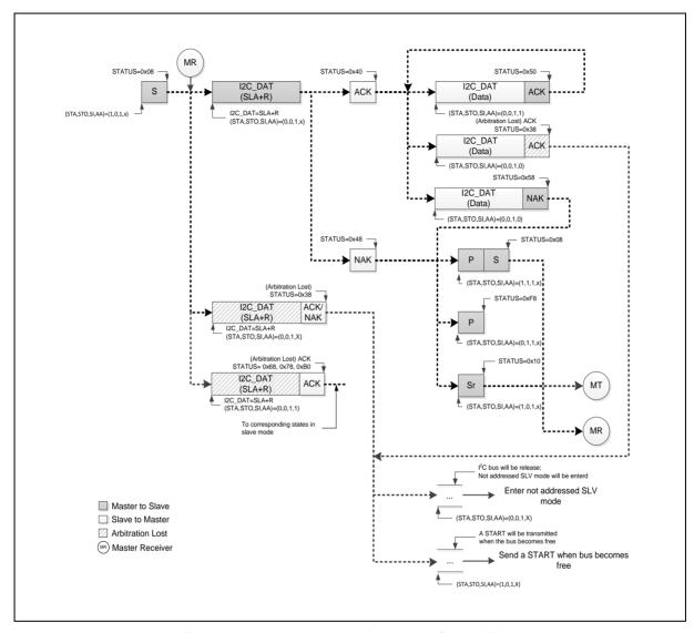
Figure 6.16-13 Master Receiver Mode Control Flow
