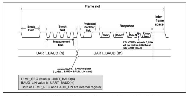
Figure 6.14-24 UART\_BAUD Update Sequence in AR mode if SLVDUEN is 0
