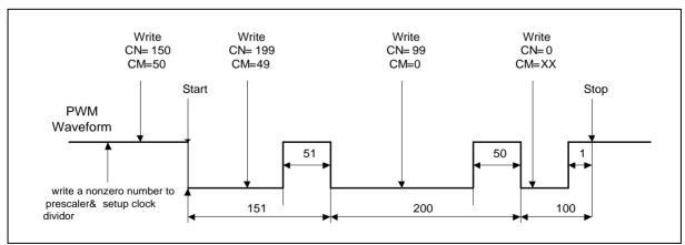
Figure 6.10-3 PWM Double Buffer Illustration
