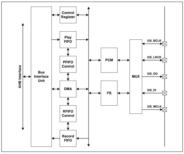
Figure 6.19-1 I<sup>2</sup>S Controller Block Diagram
