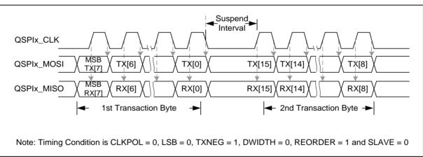
Figure 6.18-9 Timing Waveform for Byte Suspend
