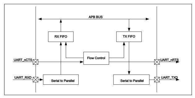
Figure 6.14-12 Auto-Flow Control Block Diagram
