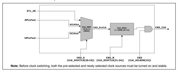
Figure 6.3-7 Reference Clock Output Divider Block Diagram
