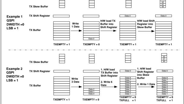
Figure 6.18-19 Transmit FIFO Buffer Example
