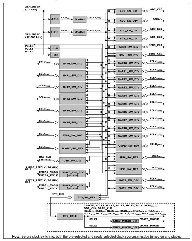
Figure 6.3-1 Clock Controller Block Diagram
