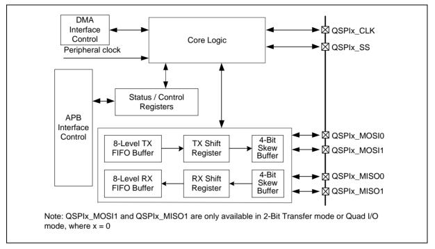
Figure 6.18-1 QSPI Block Diagram
