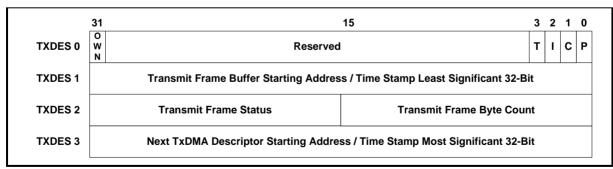
Figure 6.20-5 TXDMA Descriptor Data Structure
