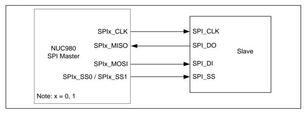
Figure 6.17-3 SPI Full-Duplex Master Mode Application Block Diagram
