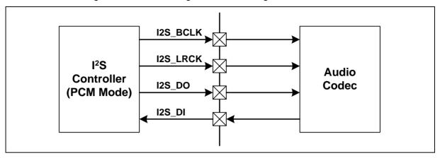
Figure 6.19-5 PCM Mode Signal Interface
