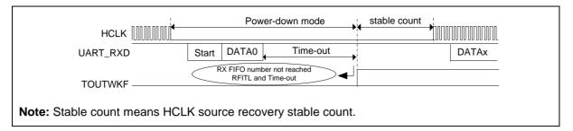
Figure 6.14-11 UART Received Data FIFO threshold time-out wake-up
