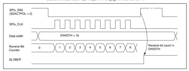
Figure 6.17-16 Slave Mode Bit Count Error
