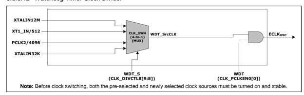
Figure 6.3-12 Watchdog Timer Clock Divider Block Diagram
