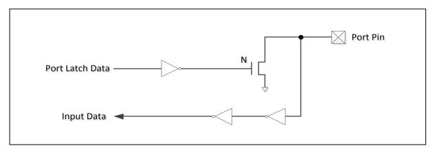
Figure 6.7-3 Open-Drain Output
