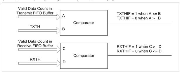
Figure 6.18-18 FIFO Threshold Comparator
