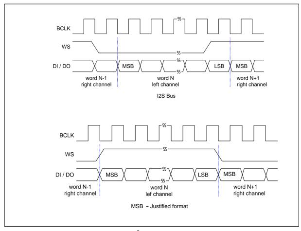
Figure 6.19-4 I<sup>2</sup>S MSB-Justified Format
