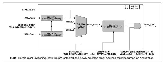
Figure 6.3-9 CMOS Sensor Controller Divider Block Diagram
