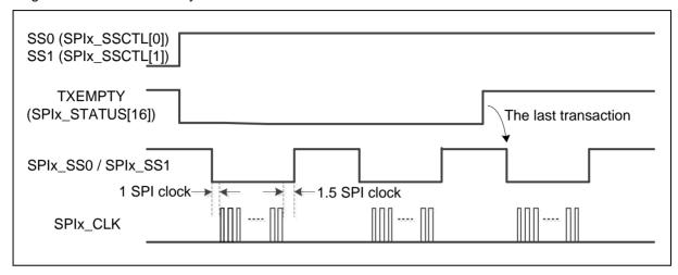
Figure 6.17-6 Automatic Slave Selection (SSACTPOL = 0, SUSPITV > 0x2)
