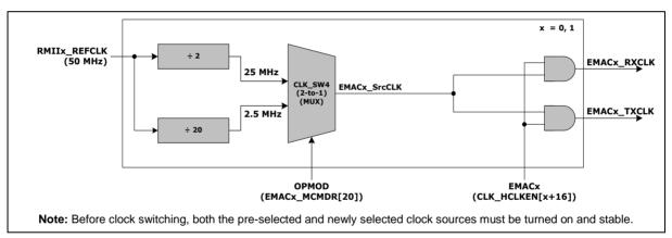
Figure 6.3-5 Ethernet MAC Controller Clock Divider Block Diagram
