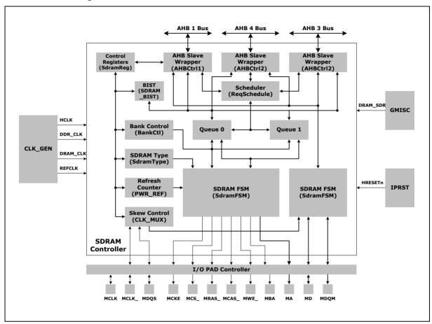
Figure 6.5-1 SDRAM Controller Block Diagram
