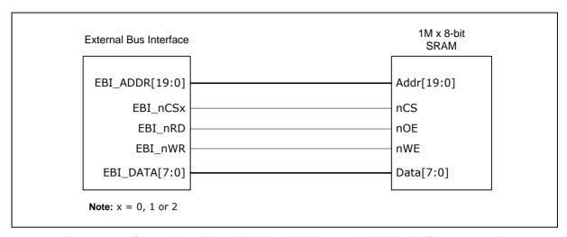
Figure 6.6-3 Connection of 8-bit EBI Data Width with 8-bit Device in Separate mode
