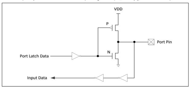
Figure 6.7-2 Push-Pull Output
