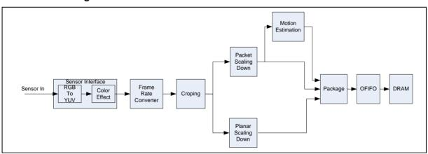
Figure 6.27-1 Image Capture Functional Block Diagram
