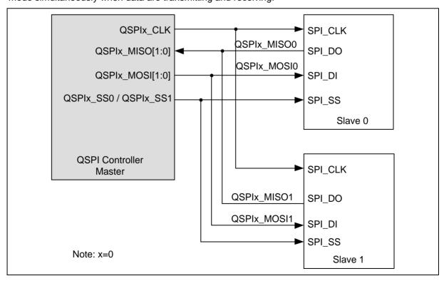
Figure 6.18-12 Two-bit Transfer Mode System Architecture
