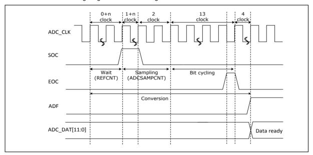
Figure 6.28-4 ADC Timing Diagram
