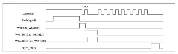
Figure 6.16-21 I<sup>2</sup>C Wake-Up Related Signals Waveform
