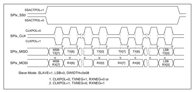
Figure 6.17-19 SPI Timing in Slave Mode
