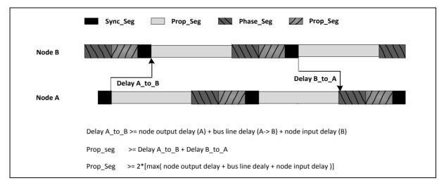
Figure 6.23-8 Propagation Time Segment
