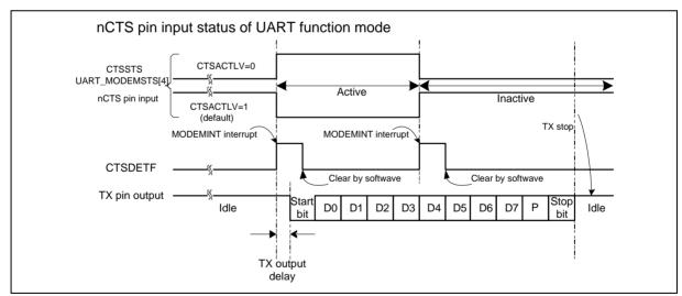
Figure 6.14-13 UART nCTS Auto-Flow Control Enabled
