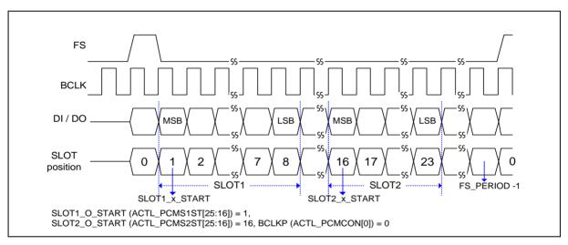
Figure 6.19-6 PCM Mode Interface Waveform
