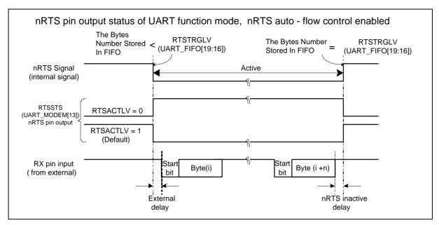
Figure 6.14-14 UART nRTS Auto-Flow Control Enabled
