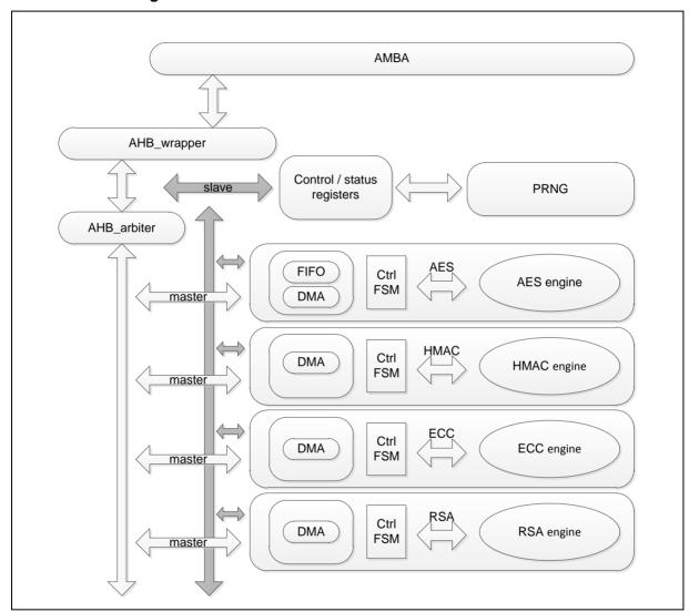
Figure 6.26-1 Cryptographic Accelerator Block Diagram
