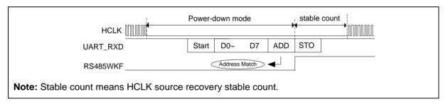
Figure 6.14-10 UART RS-485 AAD Mode Address Match Wake-up
