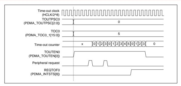
Figure 6.8-6 Example of PDMA Channel 0 Time-out Counter Operation
