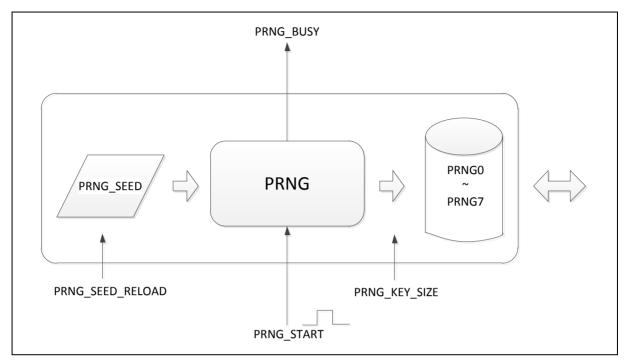
Figure 6.26-2 PRNG Function Diagram
