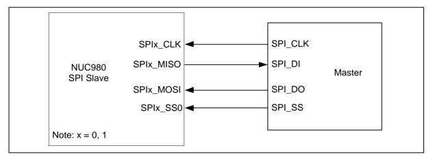
Figure 6.17-4 SPI Full-Duplex Slave Mode Application Block Diagram
