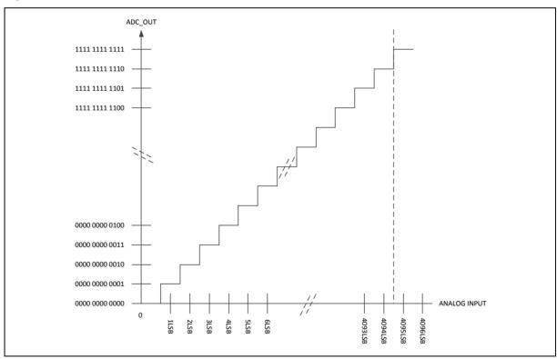
Figure 6.28-2 ADC Transfer Function
