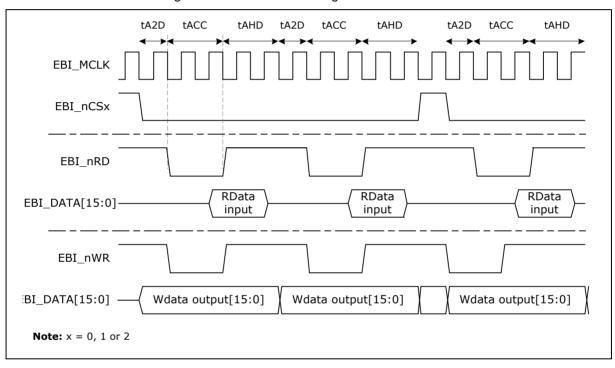
Figure 6.6-6 Timing Control Waveform for Continuous Data Access Mode
