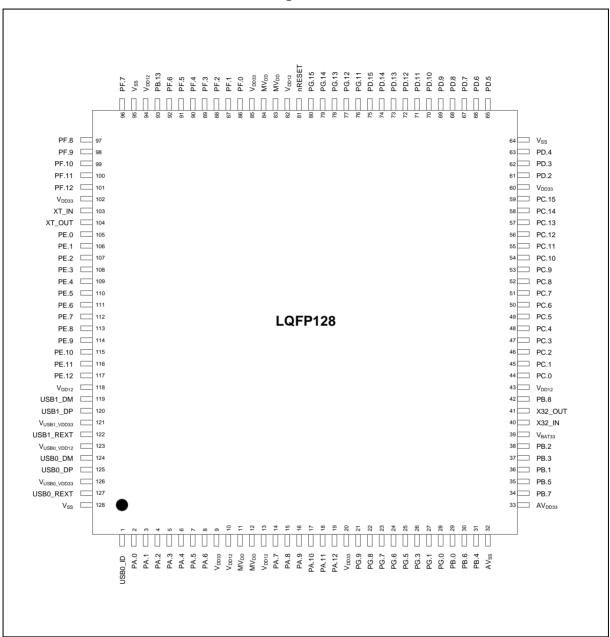
Figure 4.1-3 NUC980DKxxYC LQFP 128-pin Diagram
