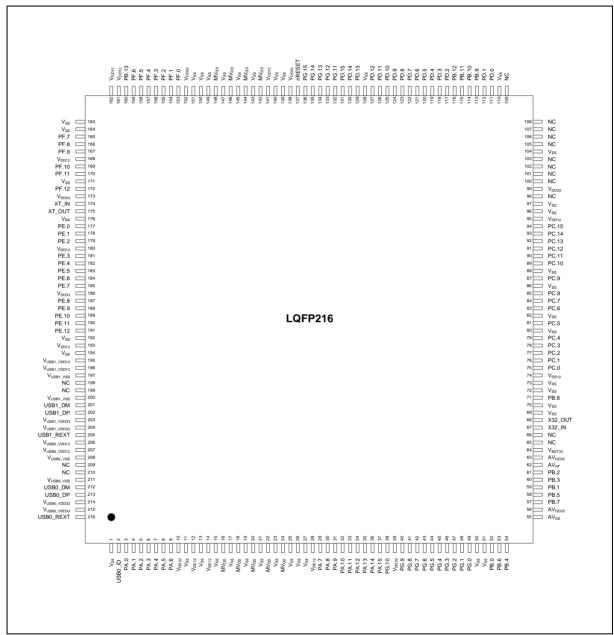
Figure 4.1-4 NUC980DFxxY LQFP 216-pin Diagram
