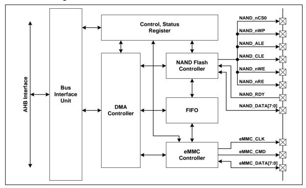
Figure 6.24-1 FMI Block Diagram
