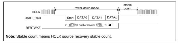
Figure 6.14-9 UART Received Data FIFO reached threshold wake-up
