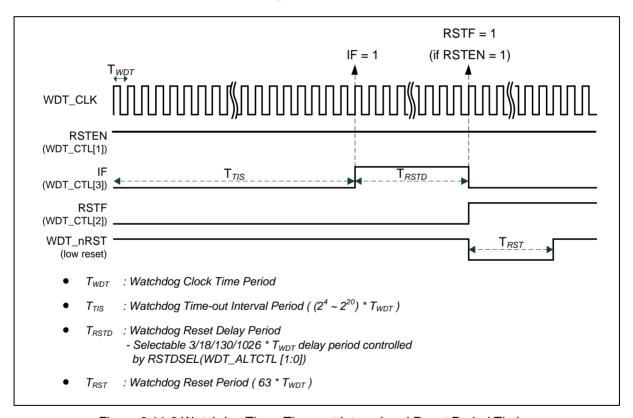
Figure 6.11-3 Watchdog Timer Time-out Interval and Reset Period Timing
