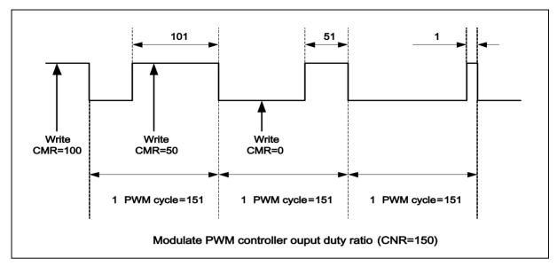
Figure 6.10-4 PWM Controller Output Duty Ratio
