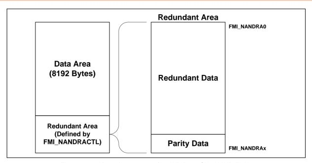
Figure 6.24-4 Data Arrangement for 8 KB Page Size NAND Flash
