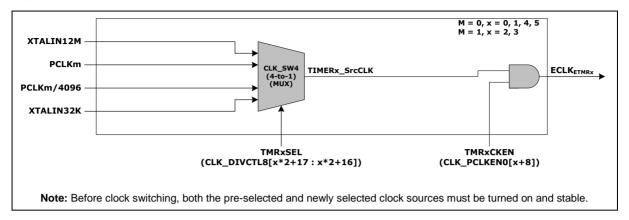
Figure 6.3-4 Timer Clock Divider Clock Diagram
