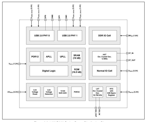
Figure 6.2-1 NUC980 Series Power Distribution Diagram
