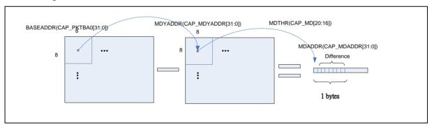
Figure 6.27-4 MDSM (MD[9]) is set to 0 and MDBS (MD[8]) is set to 1
