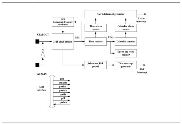
Figure 6.13-1 RTC Functional Block Diagram
