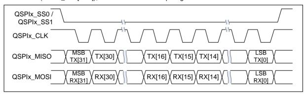
Figure 6.18-5 32-bit in One Transaction
