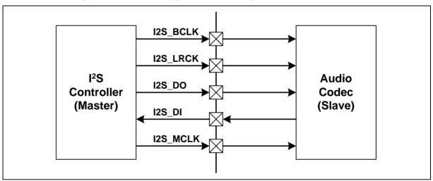
Figure 6.19-2 I<sup>2</sup>S Interface Signal of Master Mode
