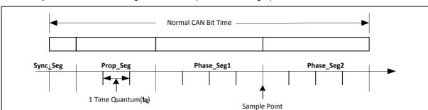
defined by the Phase Buffer Segments to compensate for edge phase errors.
