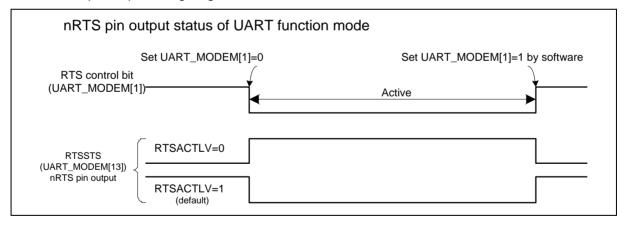
Figure 6.14-15 UART nRTS Auto-Flow with Software Control
