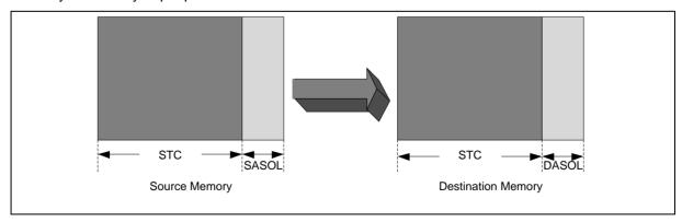
Figure 6.8-7 Stride Function Block Transfer
