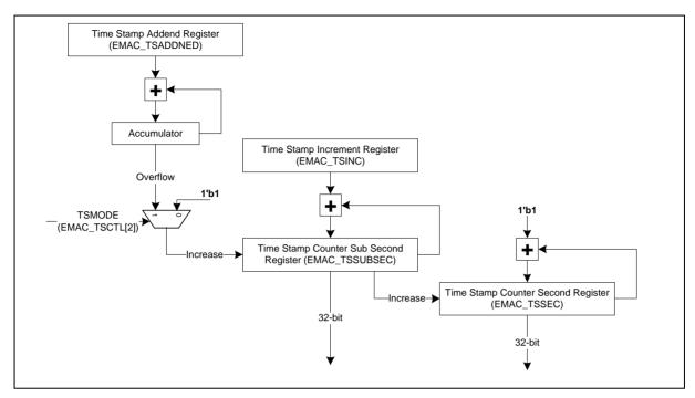
Figure 6.20-364-bit Reference Timing Counter
