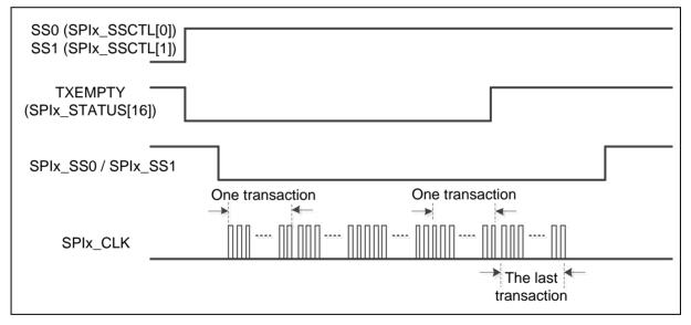
Figure 6.17-7 Automatic Slave Selection (SSACTPOL = 0, SUSPITV < 0x3)
