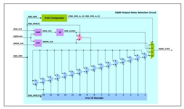
Figure 6.5-2 Clock Delay Circuit
