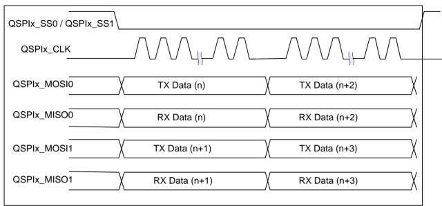
Figure 6.18-13 Two-bit Transfer Mode Timing (Master Mode)
