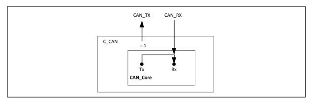
Figure 6.23-2 CAN Core in Silent Mode
