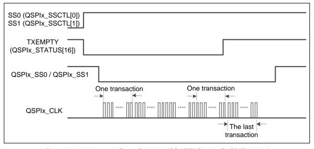
Figure 6.18-7 Automatic Slave Selection (SSACTPOL = 0, SUSPITV < 0x3)
