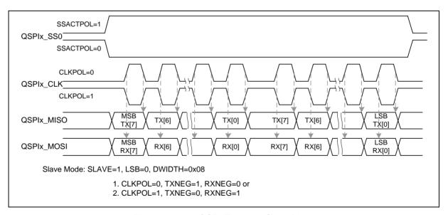
Figure 6.18-28 QSPI Timing in Slave Mode
