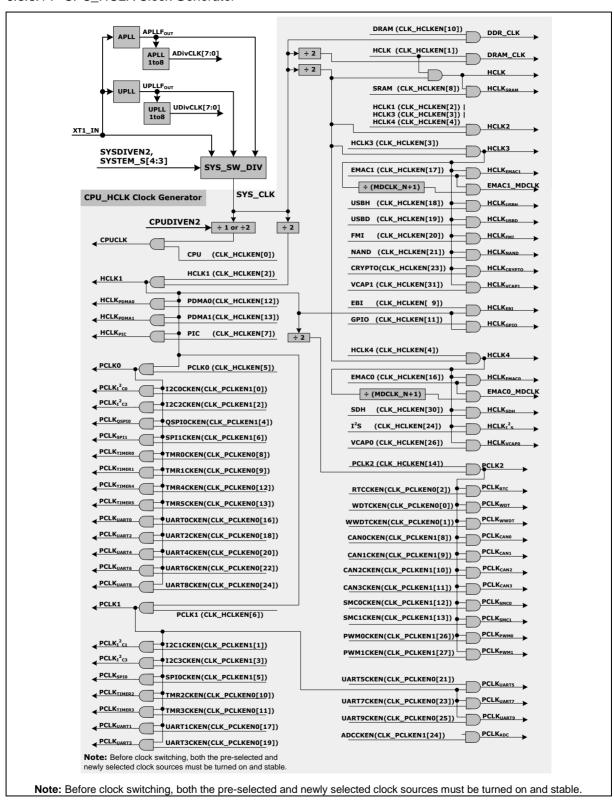
Figure 6.3-14 CPU\_HCLK Clock Generator Block Diagram
