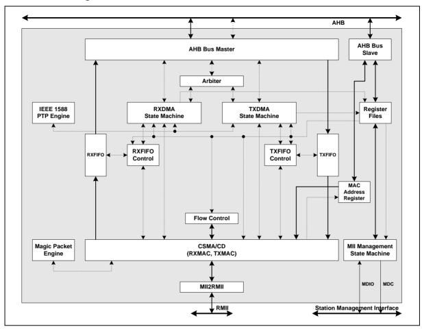
Figure 6.20-1 Ethernet MAC Controller Block Diagram
