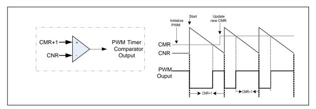
Figure 6.10-2 Legend of Internal Comparator Output of PWM-Timer
