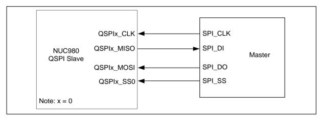
Figure 6.18-4 QSPI Full-Duplex Slave Mode Application Block Diagram
