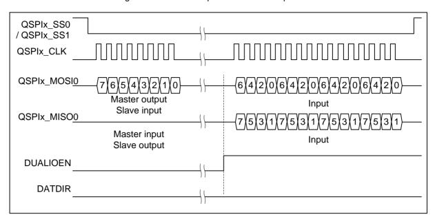
Figure 6.18-14 Bit Sequence of Dual Output Mode
