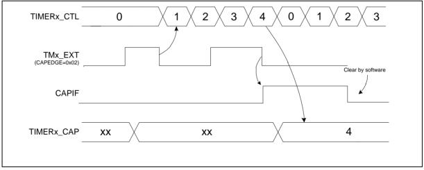
Figure 6.9-6 External CaptureTrigger-Counting Mode (CAPCNTMD (TIMERx CTL[20] is 1))
