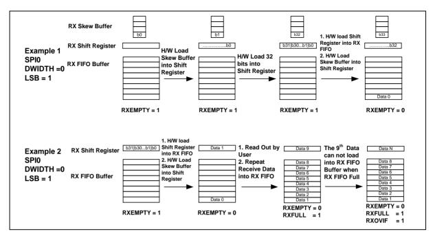
Figure 6.17-14 Receive FIFO Buffer Example
