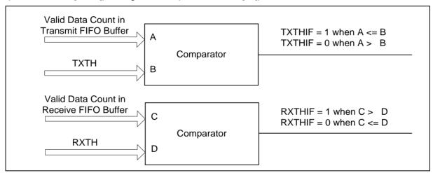
Figure 6.17-12 FIFO Threshold Comparator
