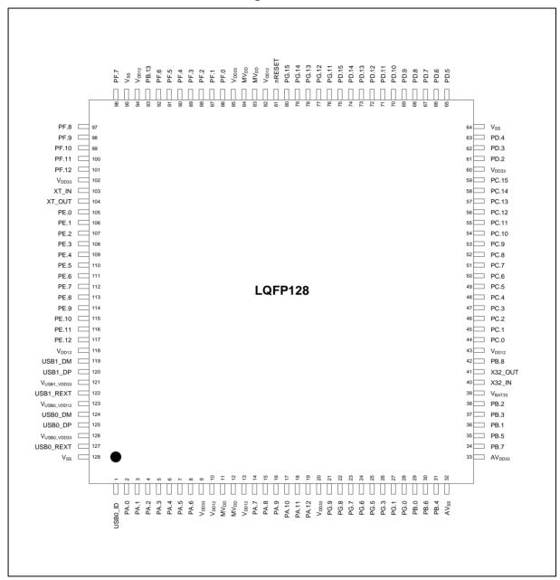
Figure 4.1-2 NUC980DKxxY LQFP 128-pin Diagram
