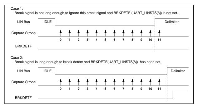
Figure 6.14-20 Break Detection in LIN Mode
