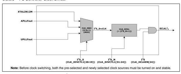
Figure 6.3-6 I<sup>2</sup>S Controller Clock Divider Block Diagram
