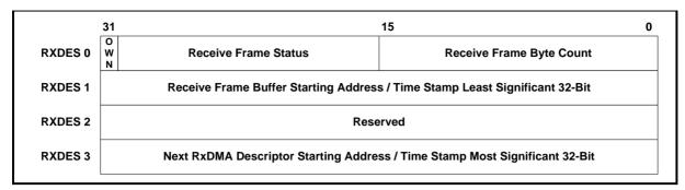
Figure 6.20-4 RXDMA Descriptor Data Structure
