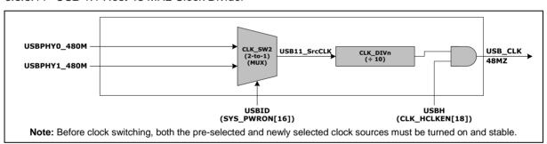
Figure 6.3-11 USB 1.1 Host Controller 48 MHz Clock Divider Block Diagram
