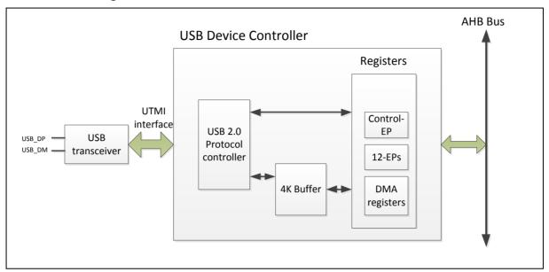
Figure 6.21-1 USB Device Controller Block Diagram
