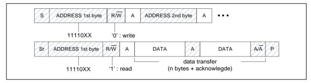
Figure 6.16-10 Master Reads Data from Slave by 10-bit
