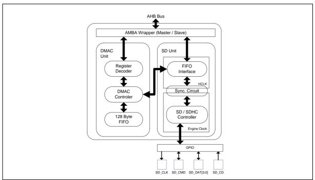
Figure 6.25-1 SD Host Controller Block Diagram
