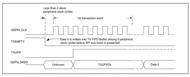
Figure 6.18-23 TX Underflow Event (QSPI0 Slave 3-Wire Mode Enabled)
