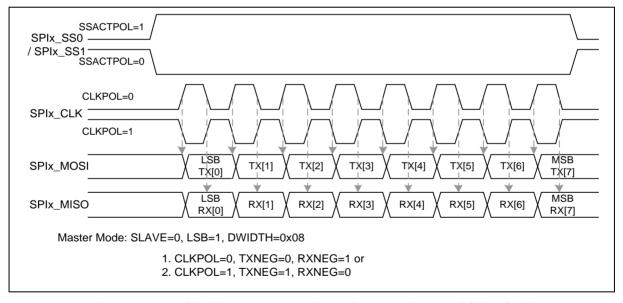
Figure 6.17-18 SPI Timing in Master Mode (Alternate Phase of SPIx\_CLK)
