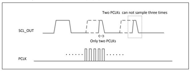
Figure 6.16-17 Setup Time Wrong Adjustment
