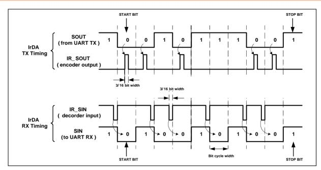
Figure 6.14-17 IrDA TX/RX Timing Diagram
