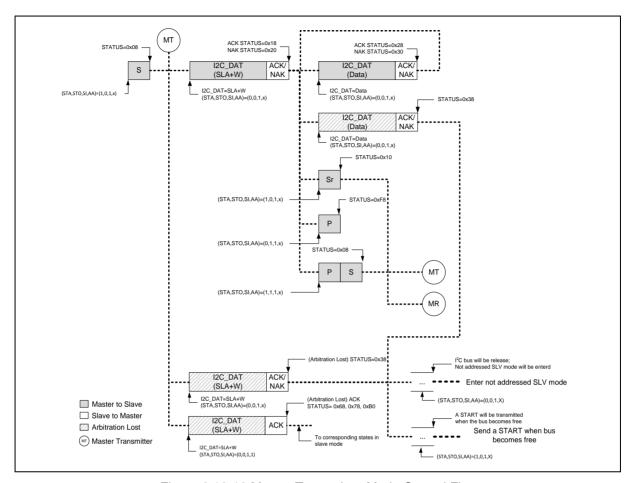
Figure 6.16-12 Master Transmitter Mode Control Flow
