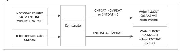
Figure 6.12-3 WWDT Reset and Reload Behavior
