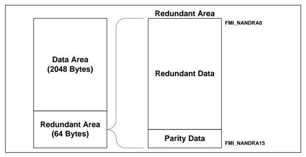
Figure 6.24-2 Data Arrangement for 2 kB Page Size NAND Flash
