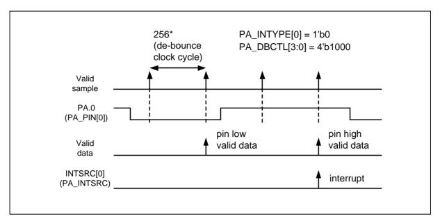
Figure 6.7-4 GPIO Rising Edge Trigger Interrupt
