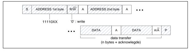
Figure 6.16-9 Master Transmits Data to Slave by 10-bit
