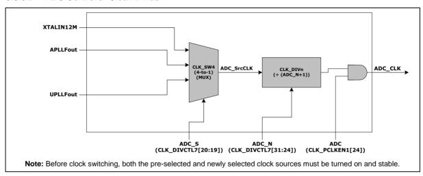
Figure 6.3-2 ADC Controller Clock Divider Block Diagram
