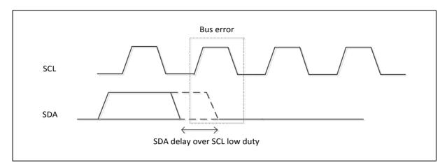
Figure 6.16-18 Hold Time Wrong Adjustment
