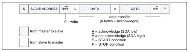
Figure 6.16-7 Master Transmits Data to Slave by 7-bit
