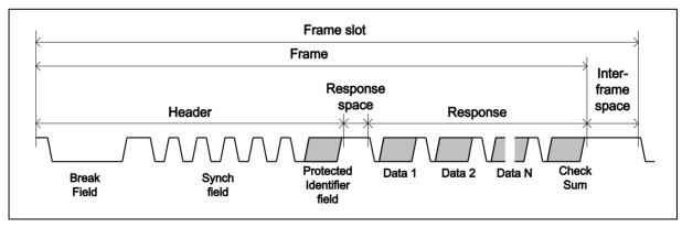
Figure 6.14-18 Structure of LIN Frame
