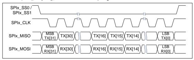
Figure 6.17-532-bit in One Transaction
