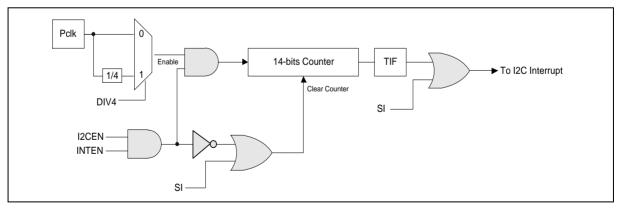
Figure 6.16-20 I<sup>2</sup>C Time-out Count Block Diagram
