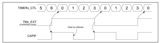
Figure 6.9-7 External CaptureReset Counter Mode (CAPCNTMD (TIMERx CTL[20] is 0))
