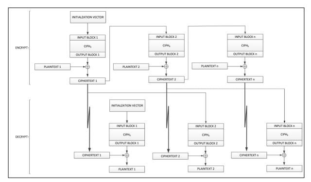
Figure 6.26-5 Cipher Feedback Mode
