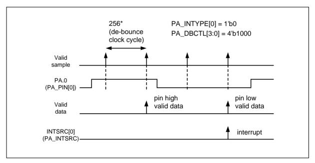
Figure 6.7-5 GPIO Falling Edge Trigger Interrupt
