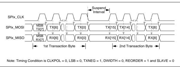
Figure 6.17-9 Timing Waveform for Byte Suspend
