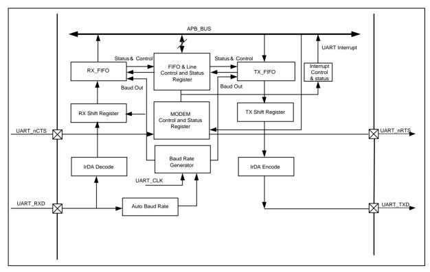
Figure 6.14-3 UART Block Diagram
