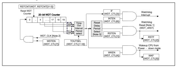
Figure 6.11-1 Watchdog Timer Block Diagram
