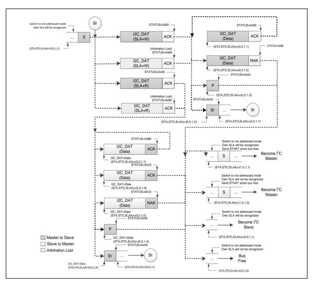
Figure 6.16-14 Slave Mode Control Flow
