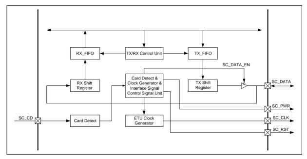
Figure 6.15-2 SC Controller Block Diagram
