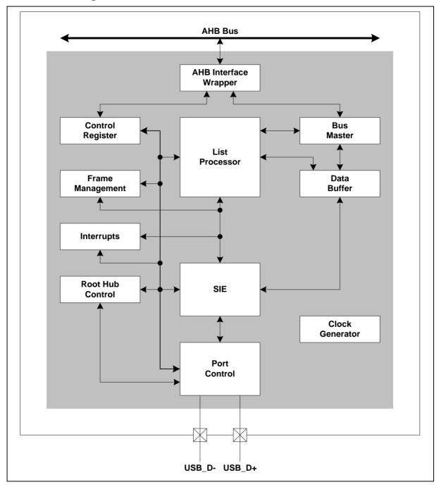
Figure 6.22-1 USB 2.0 FS Host Controller Block Diagram
