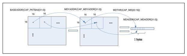
Figure 6.27-5 MDSM (MD[9]) is set to 1 and MDBS (MD[8]) is set to 0
