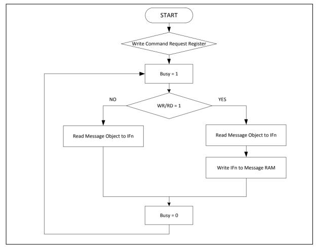
Figure 6.23-5 Data transfer between IFn Registers and Message
