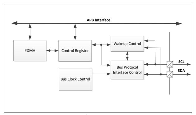
Figure 6.16-1 I<sup>2</sup>C Controller Block Diagram
