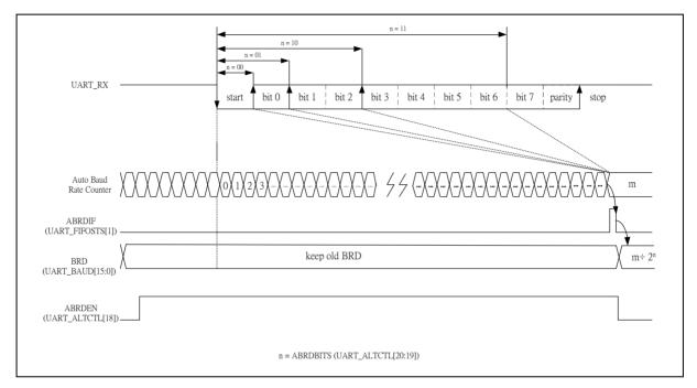
Figure 6.14-4 Auto-Baud Rate Measurement
