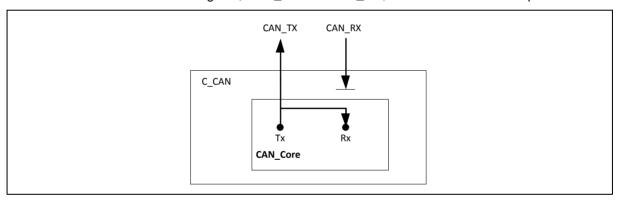
Figure 6.23-3 CAN Core in Loop Back Mode
