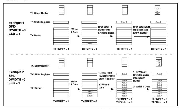
Figure 6.17-13 Transmit FIFO Buffer Example
