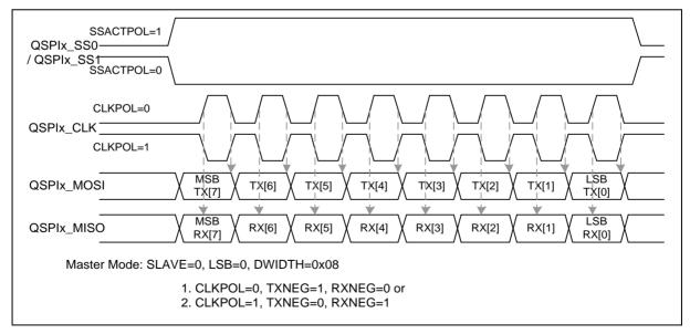
Figure 6.18-26 QSPI Timing in Master Mode
