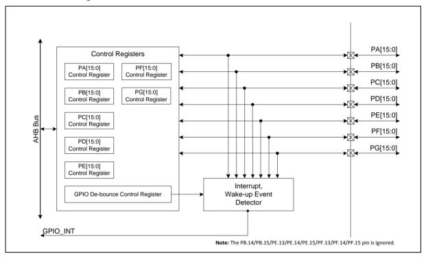
Figure 6.7-1 GPIO Block Diagram
