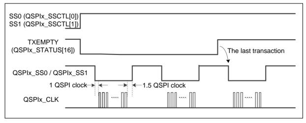
Figure 6.18-6 Automatic Slave Selection (SSACTPOL = 0, SUSPITV > 0x2)
