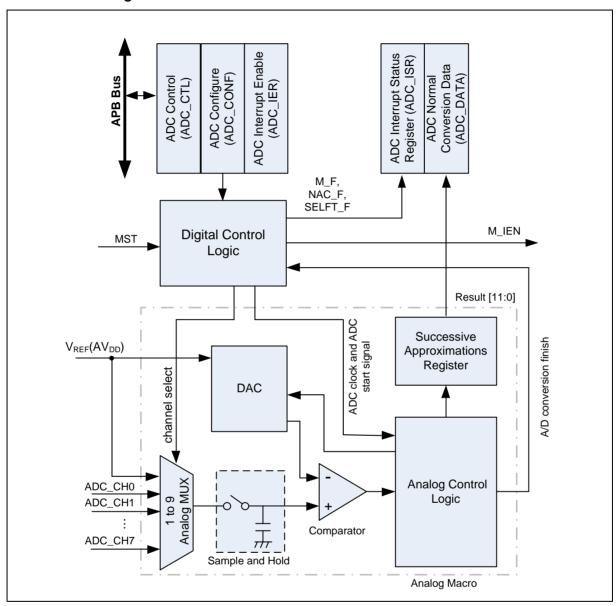
Figure 6.28-1 ADC Functional Block Diagram
