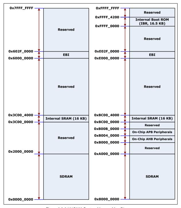
Figure 6.2-2 NUC980 System Memory Map Diagram
