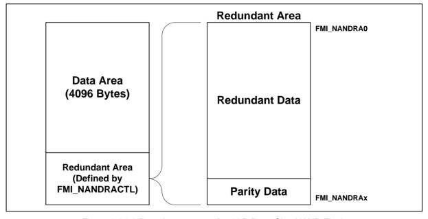
Figure 6.24-3 Data Arrangement for 4 kB Page Size NAND Flash
