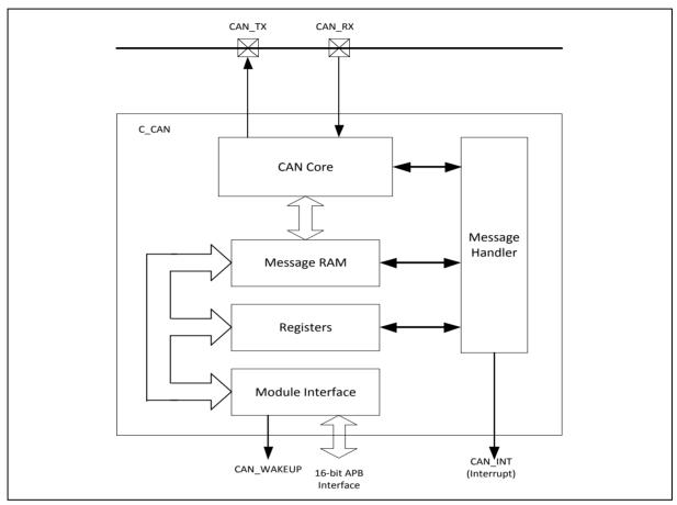
Figure 6.23-1 CAN Peripheral Block Diagram
