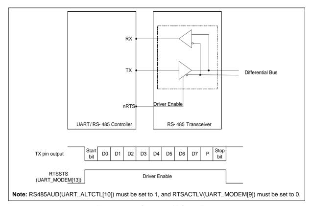
Figure 6.14-27 Structure of RS-485 Frame
