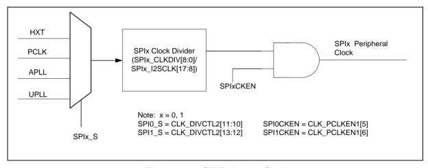
Figure 6.17-2 SPI Peripheral Clock
