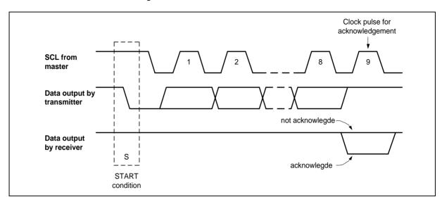
Figure 6.16-5 Bit Transfer on the I<sup>2</sup>C Bus
