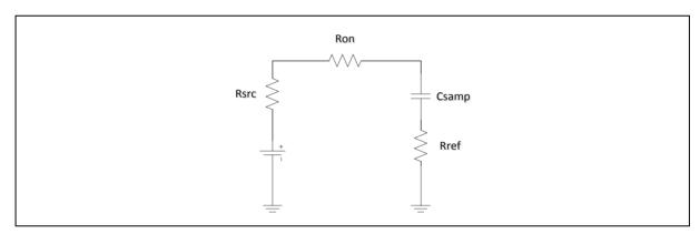
Figure 6.28-3 Simplified Sampling Diagram
