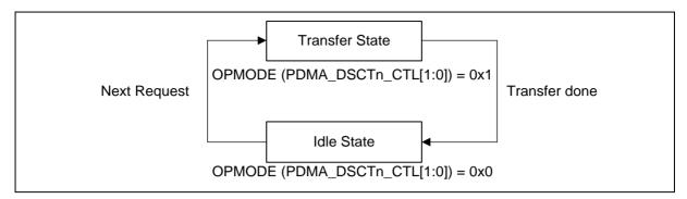
Figure 6.8-2 Basic Mode Finite State Machine
