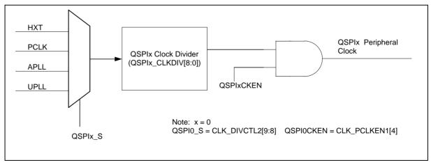
Figure 6.18-2 QSPI Peripheral Clock
