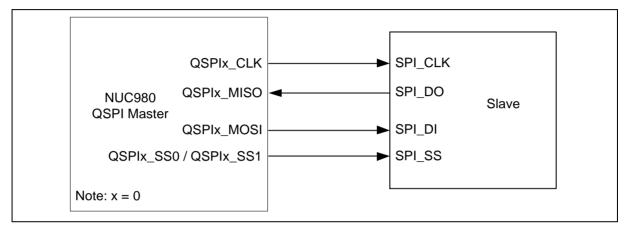
Figure 6.18-3 QSPI Full-Duplex Master Mode Application Block Diagram
