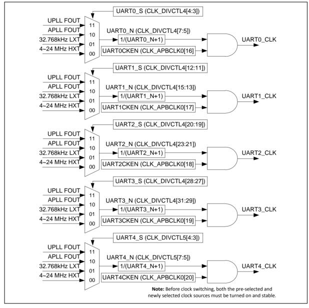
Figure 6.14-1 UART0-UART4 Clock Control Diagram
