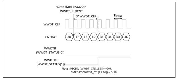
Figure 6.12-4 WWDT Reload Counter When CNTDAT > CMPDAT
