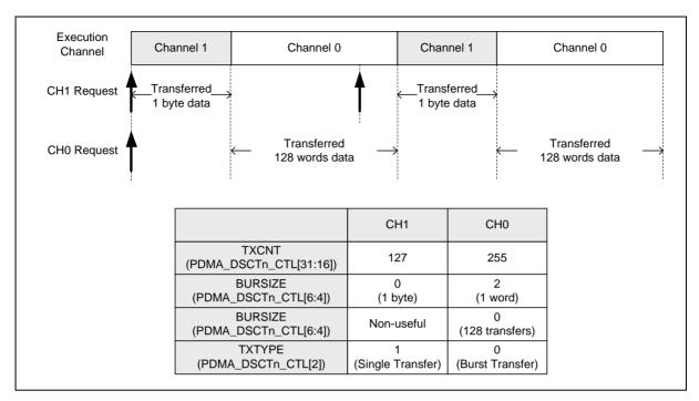
Figure 6.8-5 Example of Single Transfer Type and Burst Transfer Type in Basic Mode
