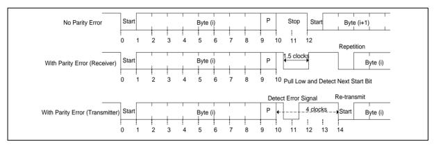
Figure 6.15-9 SC Error Signal
