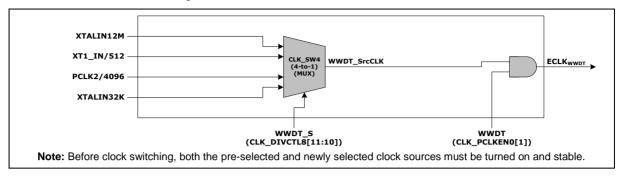
Figure 6.3-13 Windowed Watchdog Timer Clock Divider Block Diagram
