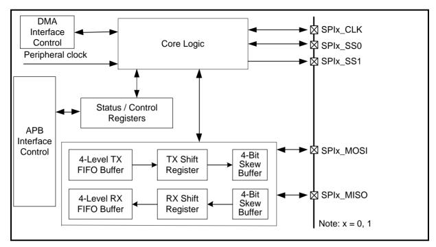
Figure 6.17-1 SPI Block Diagram
