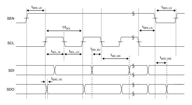
Fig.2.4.1 SPI Timing
