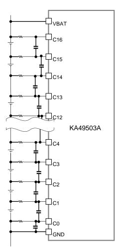
Fig.2.1.1 KA49503A Cell Connection example with 15 cell connected
