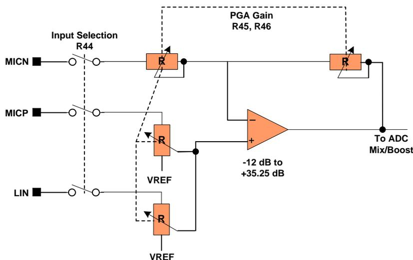
Figure 2: PGA Input Structure Simplified Schematic
