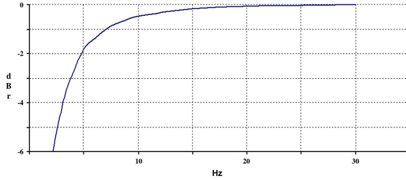
Figure 41: ADC Highpass Filter Response, Audio Mode
