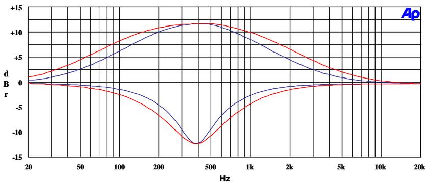
Figure 47: EQ Band 2, EQ2BW = 0 versus EQ2BW = 1
