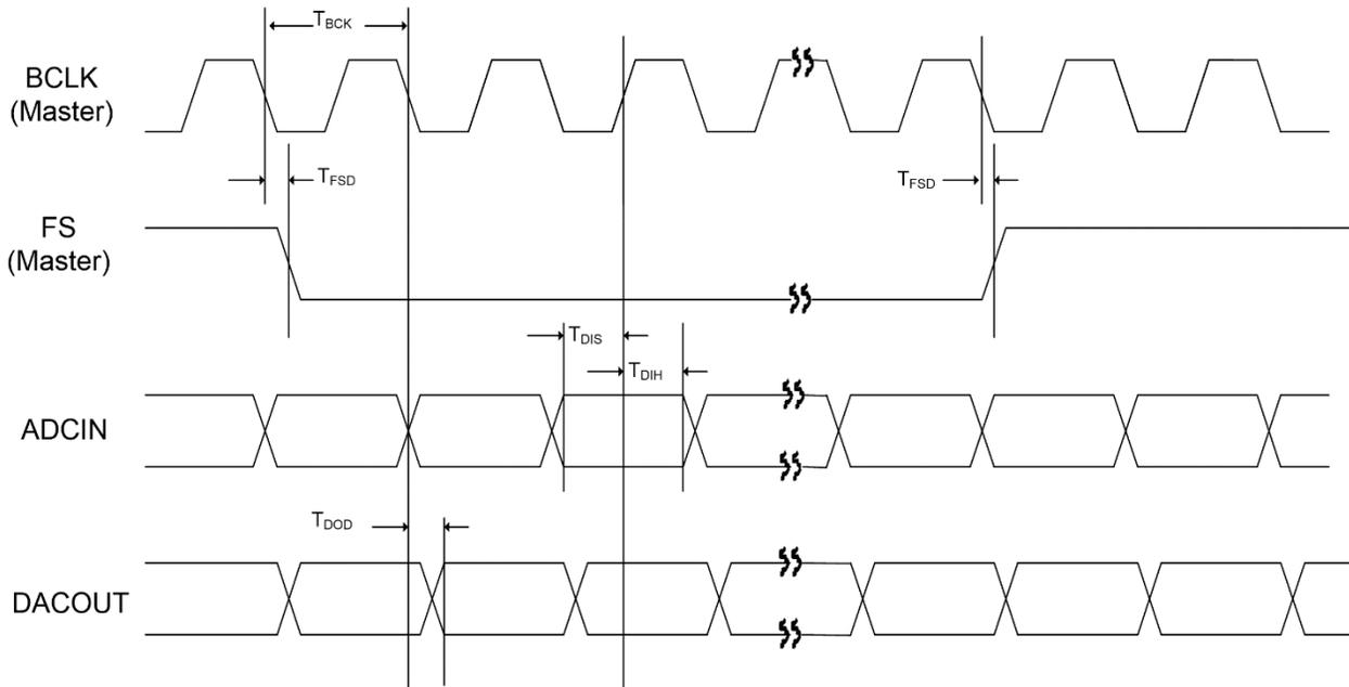
Figure 22: Digital Audio Interface Master Mode Timing
