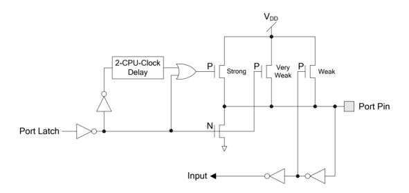
Figure 8.1. Quasi-Bidirectional Mode Structure
