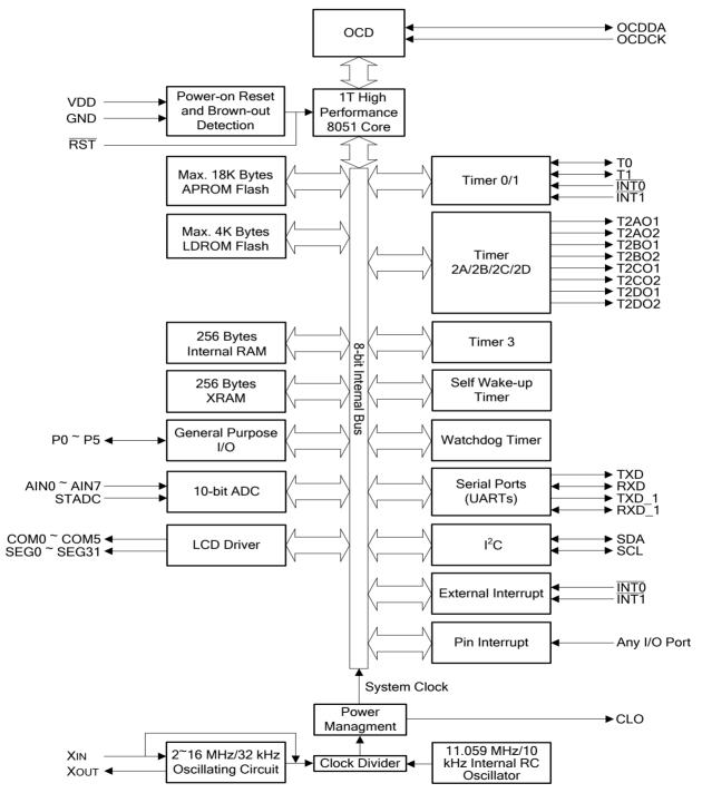
Figure 3.1. Function Block Diagram
