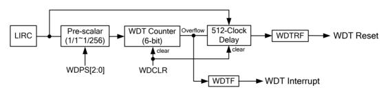
Figure 12.1. WDT as A Time-Out Reset Timer
