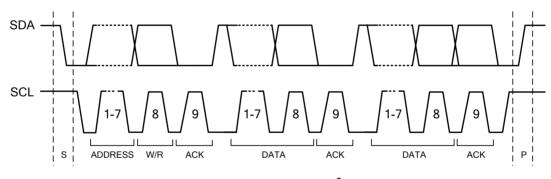
Figure 15.4. Data Format of One I<sup>2</sup>C Transfer
