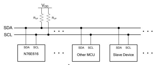
Figure 15.1. I<sup>2</sup>C Bus Interconnection
