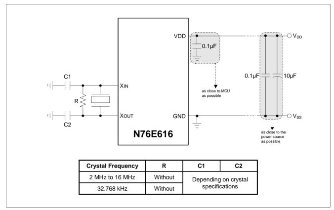
Figure 4.4. Application Circuit with External Crystal
