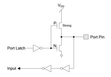
Figure 8.2. Push-Pull Mode Structure
