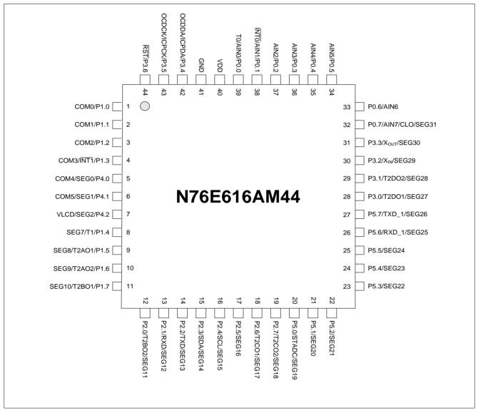
Figure 4.3 Pin Assignment of LQFP-44 Package
