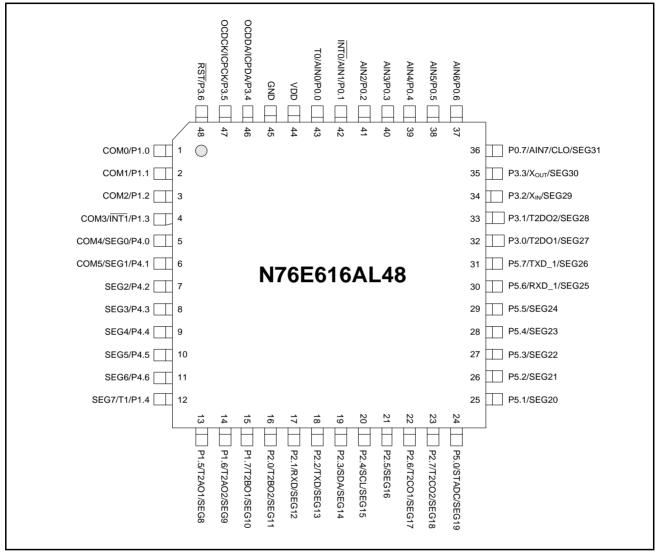
Figure 4.1. Pin Assignment of LQFP-48 Package
