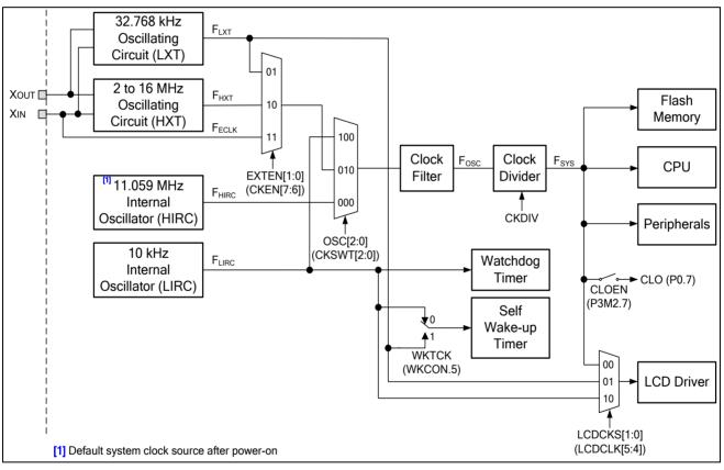
Figure 23.1 Clock System Block Diagram
