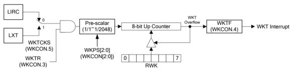
Figure 13.1. Self Wake-Up Timer Block Diagram
