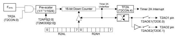
Figure 10.1. Timer 2A Auto-Reload Mode Block Diagram
