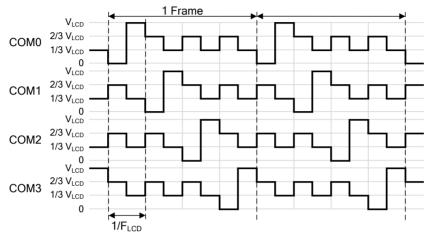
Figure 18.1. COM Driving Signals (1/4 Duty and 1/3 Bias)
