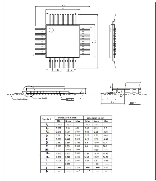
Figure 32.2 PQFP44 (10x10x2.0mm, footprint 3.2mm) Package Dimension
