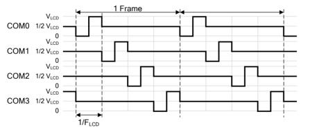
Figure 18.4. COM Driving Signals (1/4 Duty and 1/2 Bias)
