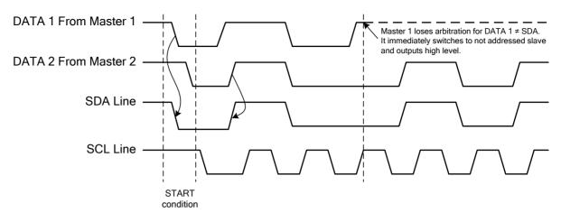
Figure 15.6. Arbitration Procedure of Two Masters
