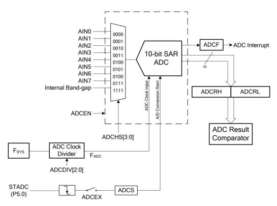
Figure 17.1. 10-bit ADC Block Diagram
