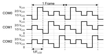
Figure 18.2. COM Driving Signals (1/3 Duty and 1/3 Bias)
