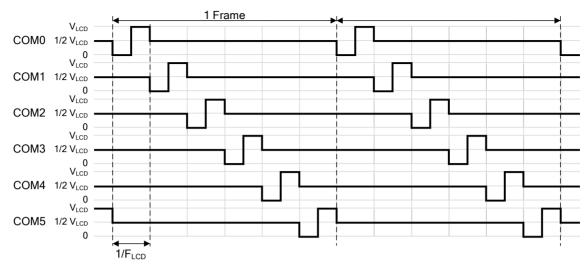
Figure 18.6. COM Driving Signals (1/6 Duty and 1/2 Bias)
