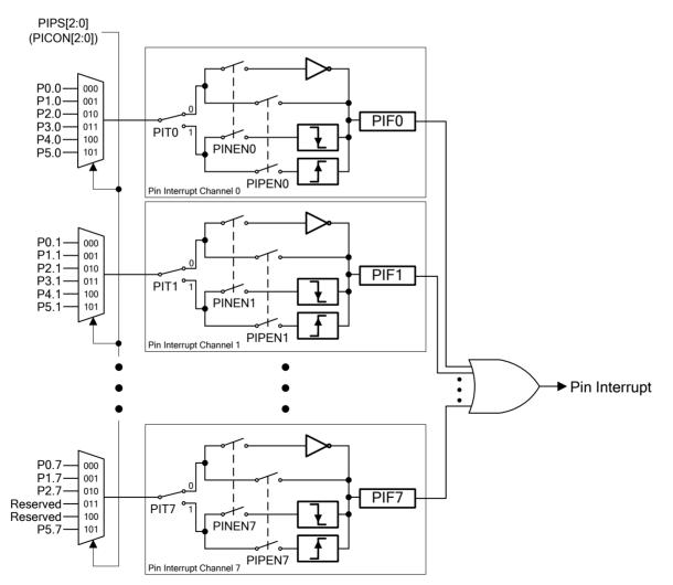
Figure 16.1. Pin Interface Block Diagram
