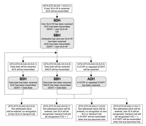
Figure 15.9. Flow and Status of Slave Receiver Mode
