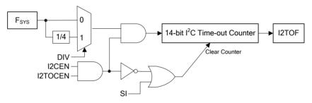
Figure 15.12. I<sup>2</sup>C Time-Out Counter
