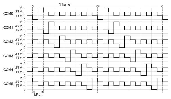
Figure 18.3. COM Driving Signals (1/6 Duty and 1/3 Bias)
