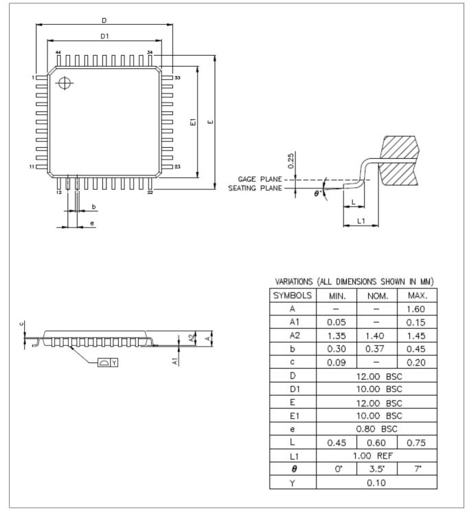
Figure 32.3 LFP44 (10x10x1.4 mm, Footprint 2.0 mm) Package Dimension
