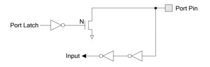
Figure 8.4. Open-Drain Mode Structure
