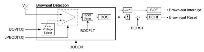
Figure 24.1. Brown-out Detection Block Diagram
