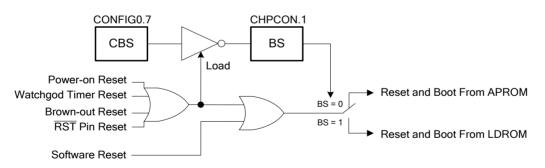
Figure 25.1. Boot Selecting Diagram
