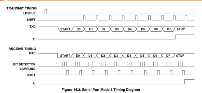
Transmission is initiated by any writing instructions to SBUF. Transmission takes place on TXD pin. First, the start bit comes out; the 8-bit data follows to be shifted out and then ends with a stop bit. After the stop bit appears, TI (SCON.1) will be set to indicate one-byte transmission complete. All bits are shifted out depending on the rate determined by the baud rate generator.
