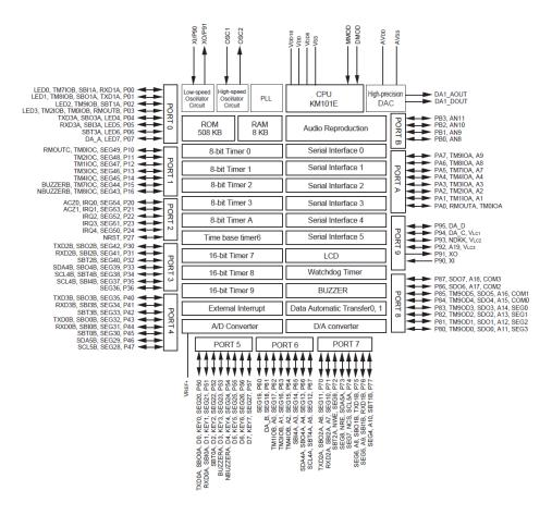
Figure: 4.1 Block Diagram
