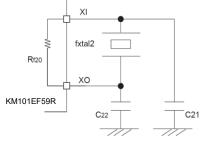
Instruction cycle becomes clock frequency divided by 1/2 Built-in feedback resistor
