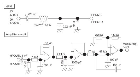
Figure: 5.7 Audio Characteristic Measuring Circuit (b)
