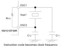
divided by 1/2 Built-in feedback resistor
