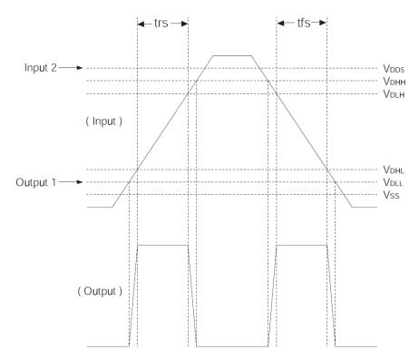
Figure: 5.5 Operation of AC Zero-Cross Detection Circuit
