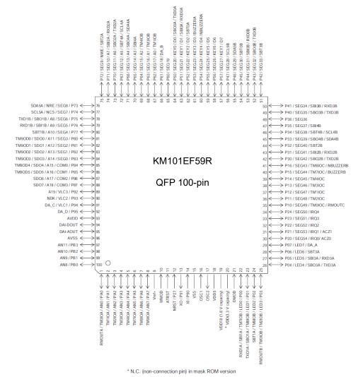
Figure: 3.1 Pin Configuration
