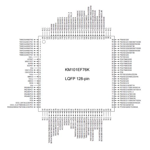
Figure: 3.1 Pin Configuration (KM101EF76K)
