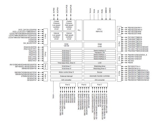
Figure: 4.2 Block Diagram (KM101EF57G)
