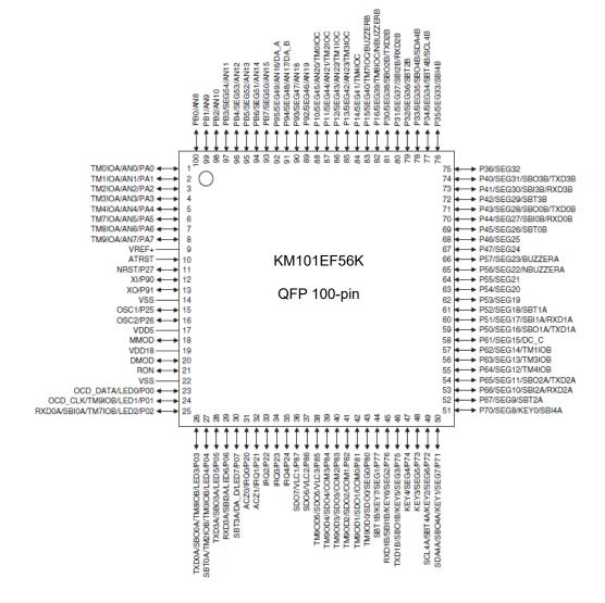
Figure: 3.3 Pin Configuration (KM101EF56K)
