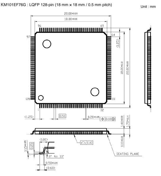
Figure: 6.1 LQFP 128-pin Package Dimension
