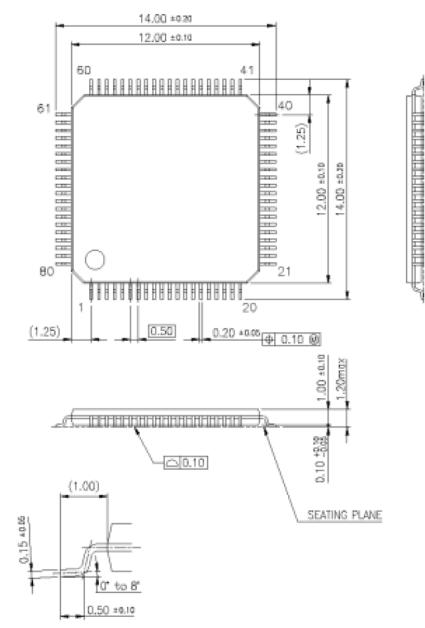
■ KM101EF57G : TQFP 80-pin (12 mm × 12 mm / 0.5 mm pitch)
