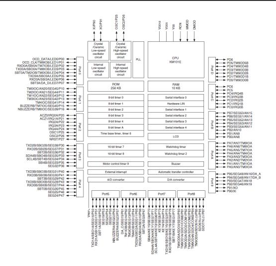
Figure: 4.1 Block Diagram (KM101EF76K)
