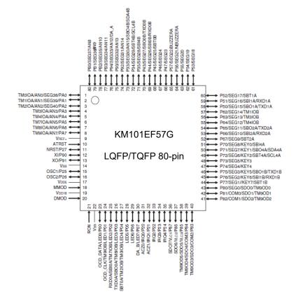
Figure: 3.2 Pin Configuration (KM101EF57G)
