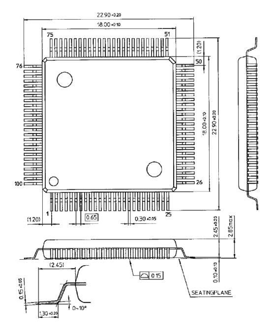
Figure: 6.4 QFP 100-pin Package Dimension
