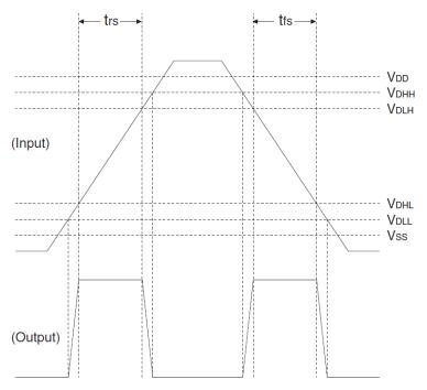
Figure: 5.6 AC zero-volt detection circuit operation
