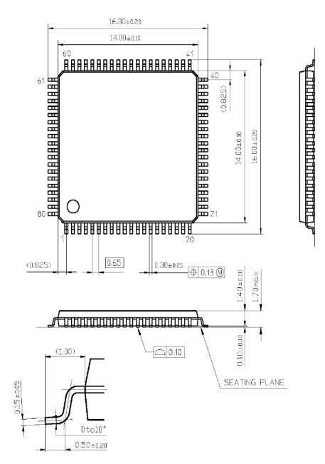
Figure: 6.2 LQFP 80-pin Package Dimension
