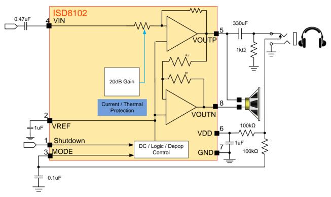
Figure 3-1 ISD8102 Earpiece Configuration Block Diagram
