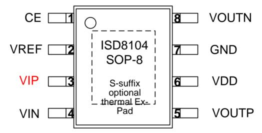
Figure 4-2 ISD8104 8-Lead SOP Pin Configuration
