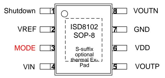
Figure 4-1 ISD8102 8-Lead SOP Pin Configuration
