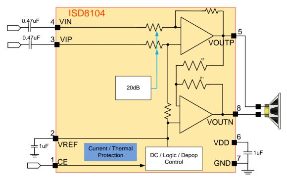
Figure 3-2 ISD8104 Differential Input Pair Block Diagram
