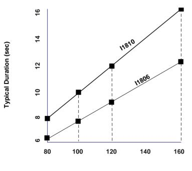
Chart 1: ISD Duration Versus  $R_{OSC}$  at  $T_A = 25^{\circ}C$  and  $V_{CC} = 3.0V$
