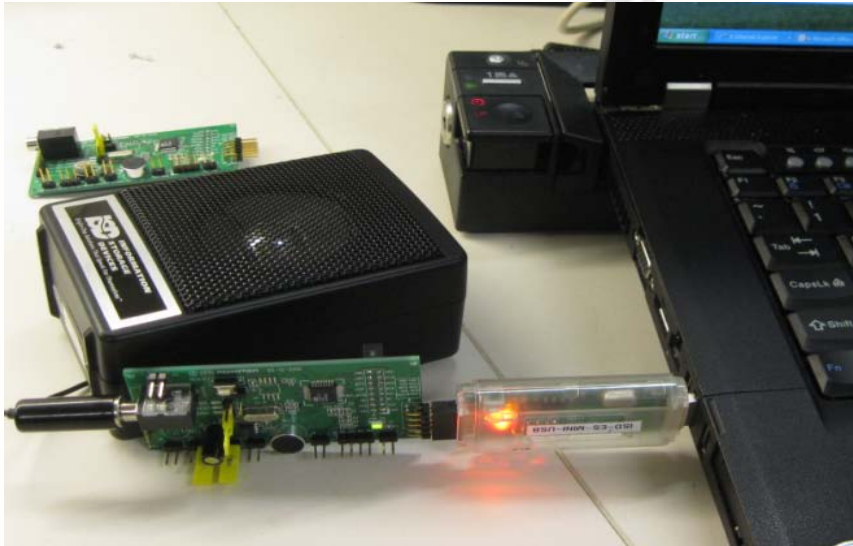
Figure 5 – A complete evaluation environment for ISD15100 device
