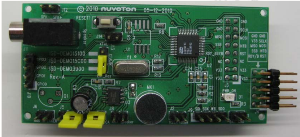
Figure 1 – Top view of ISD-DEMO15100/15C00/3900 Rev-A board
