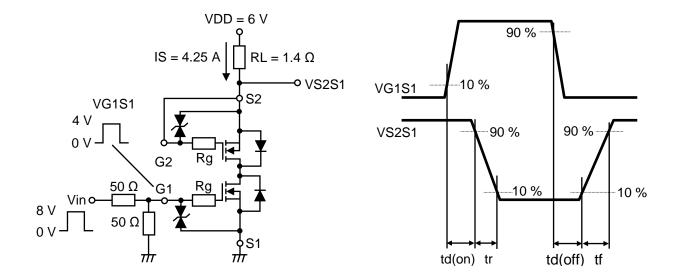
Measurement circuit for Turn-on Delay Time / Rise Time / Turn-off Delay Time / Fall Time
