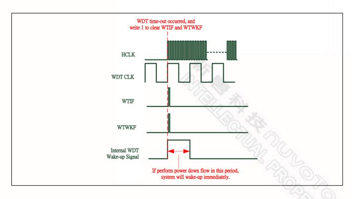
If user wants to enter Power-down mode after previous WDT time-out wake-up occurred, the user must delay one WDT peripheral clock as least to avoid entering power mode failed. For example, if the current WDT source clock is 10 kHz, the software delay time should be larger than 100 us for entering the next Power-down mode normally.
