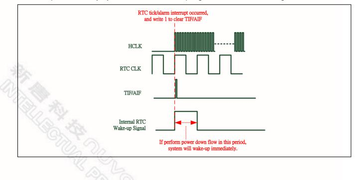
If user wants to enter Power-down mode after previous RTC wake-up event occurred, user must delay at least one RTC peripheral clock (about 30.52 us) to avoid entering power mode failed.
