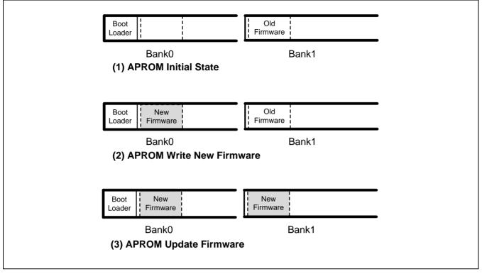
Figure 2-3 Firmware Update State in Dual Bank Flash
