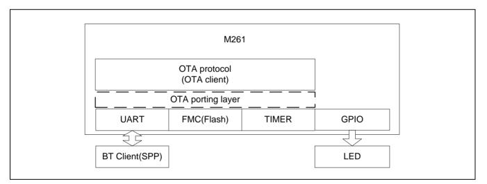
Figure 3-1 OTA Client Firmware Architecture
