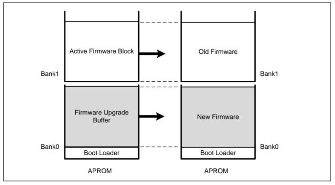
Figure 2-2 OTA Client Dual Bank Flash Diagram
