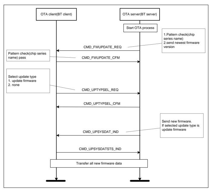
Figure 2-4 OTA Protocol Communication Flow
