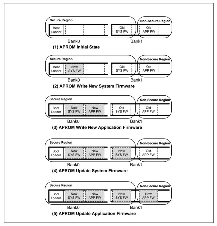
Figure 2-3 Firmware Update State in Dual Bank Flash
