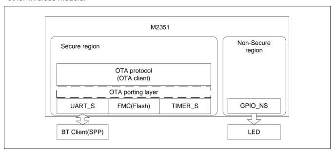
Figure 3-1 OTA Client Firmware Architecture
