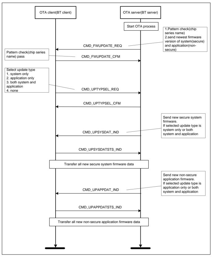
Figure 2-4 OTA Protocol Communication Flow
