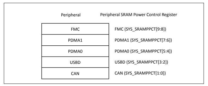
Figure 2-7 Peripheral SRAM Power Control in Power-down Mode
