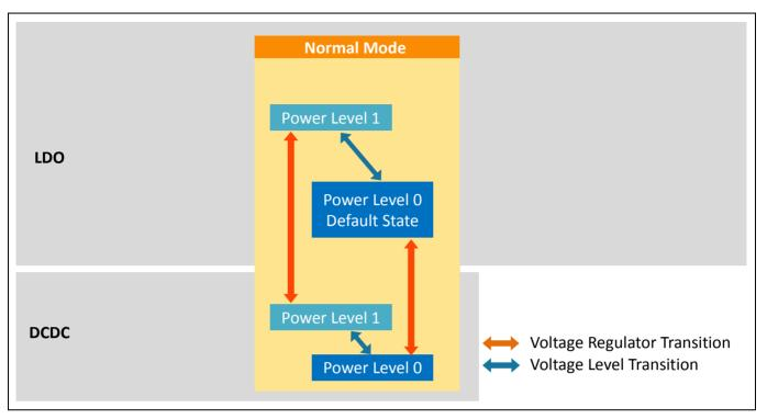
Figure 2-3 Voltage Regulator and Voltage Level Transition in Normal Mode
