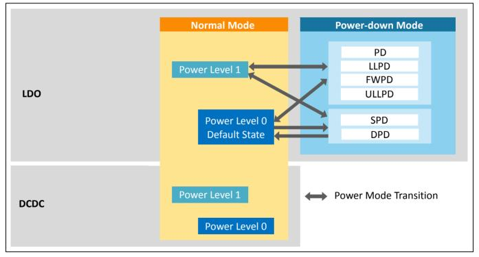
Figure 2-5 Normal Mode and Power-down Mode Transition
