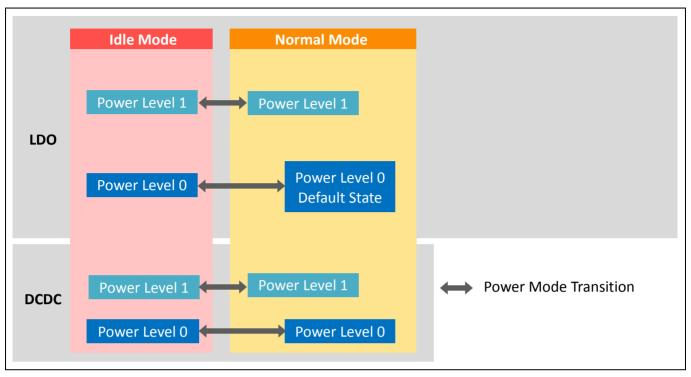
Figure 2-4 Normal Mode and Idle Mode Transition
