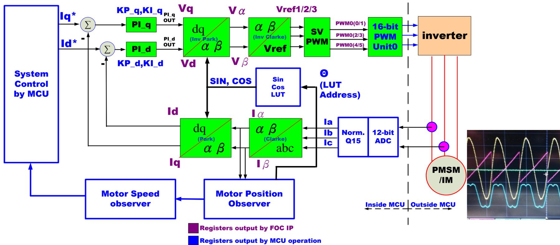
= NM1530 Series Motor-Driving Unit (MDU)
