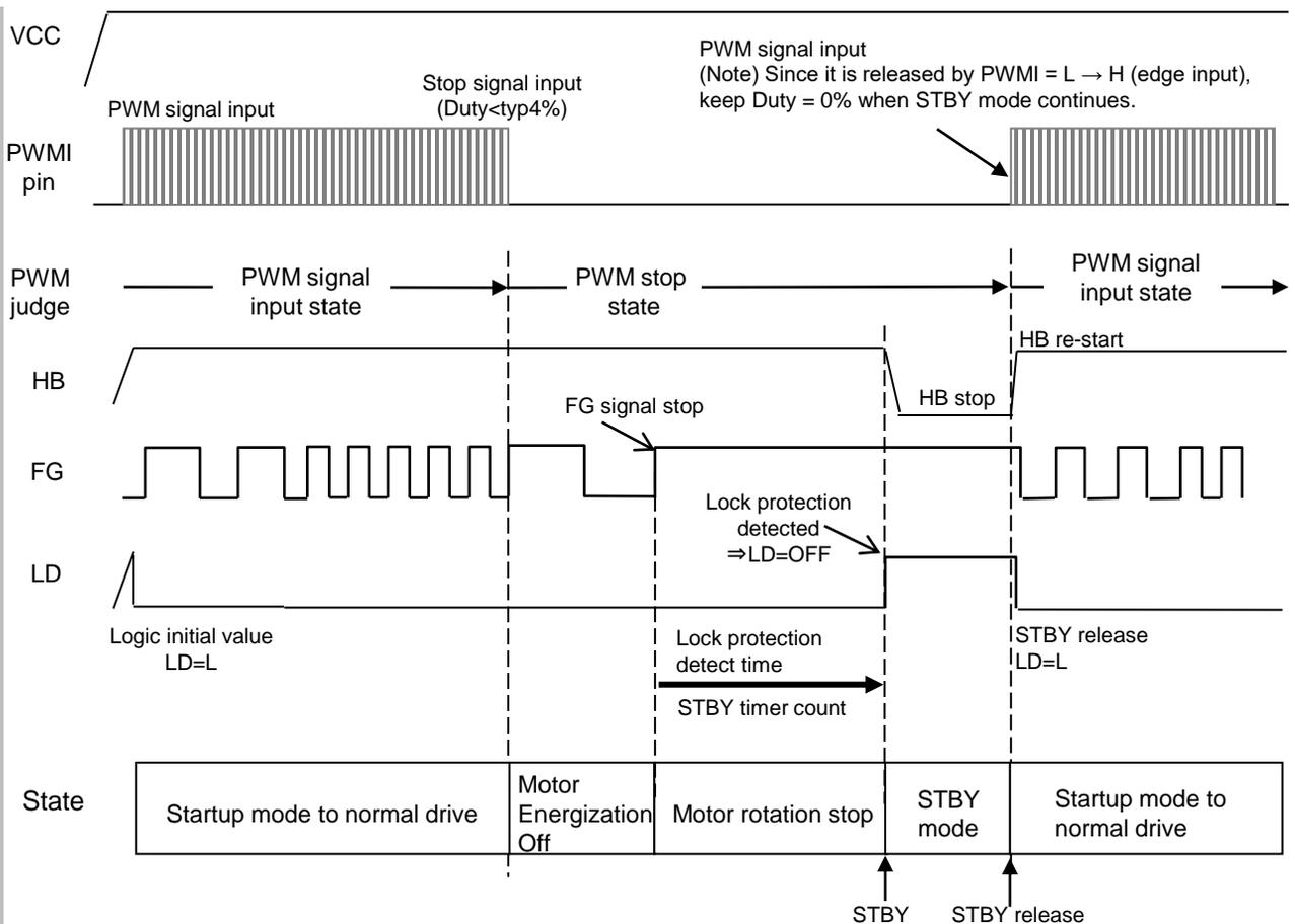
Since STBY mode is released by PWM = L → H (edge input), keep Duty = 0% when STBY mode continues. If the PWM pin is open (HiZ) in STBY mode, the STBY mode is released.
