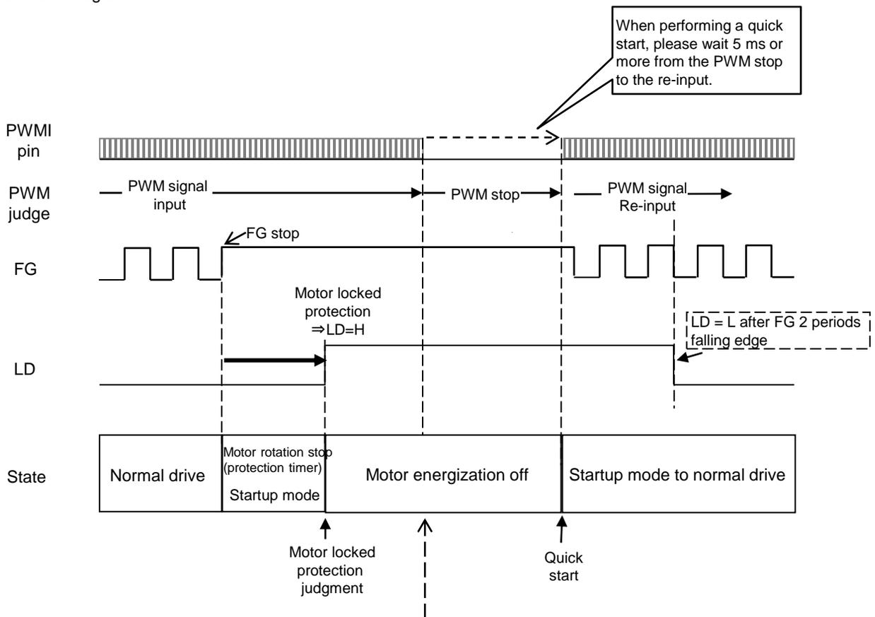
※During motor locked protection, the shift to STBY mode does not occur even after PWM stop input.
