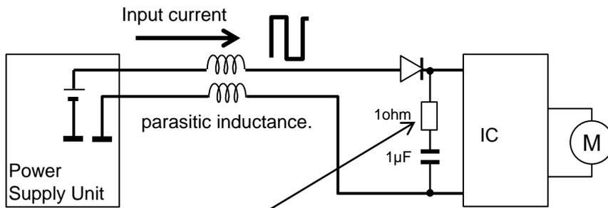
The current peak is reduces according to adding in series with bypass capacitance.
