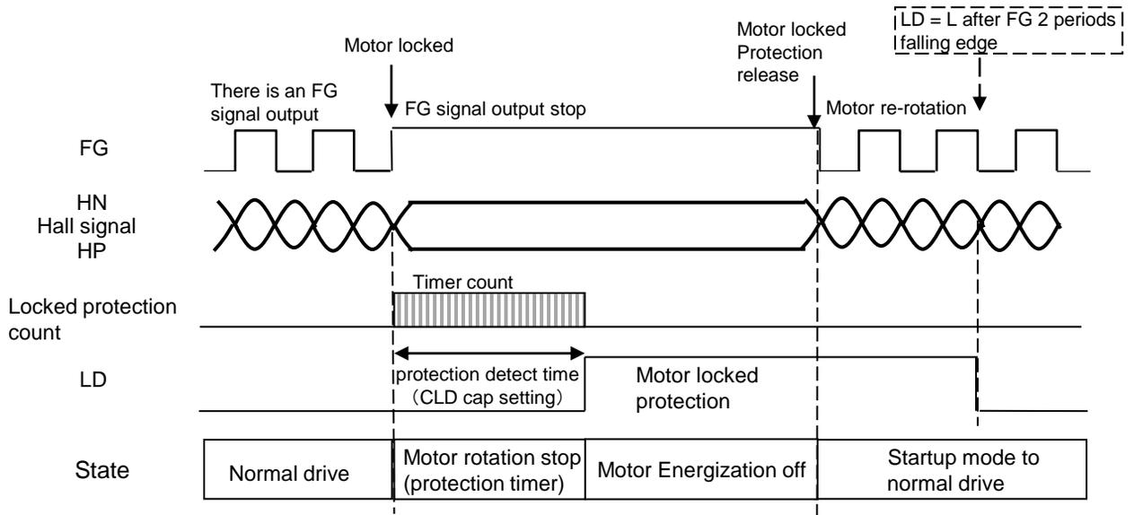
**■ Shift to the lock protection at hall signal HP < HN**
