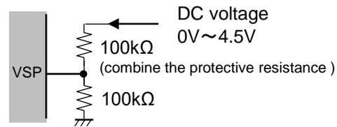
Since the resistance value is a reference value, please change according to the operating conditions. In addition, the input voltage of the VSP terminal ask attention to the absolute maximum rating. It should be noted that, If you connect a resistor to the HB terminal, please set the resistance value with attention to the rated current of the HB terminal.
